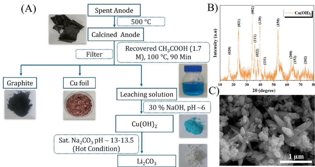
Fig. 7 (A) The flow chart for the recovery of metals and graphite from spent LIB anodes. (B) depicts the PXRD and (C) the FE-SEM of Cu(OH)<sub>2</sub> respectively.
