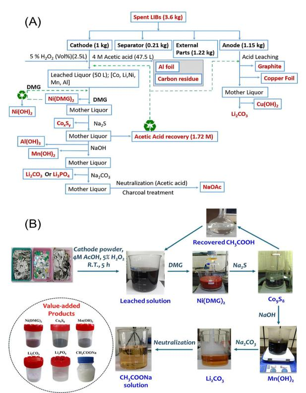
Fig. 8 (A) Flow sheet for a single batch of cathode and anode showing hydrometallurgical leaching *θ* sequential chemical precipitation methods adopted in our studies using spent LIBs, and (B) digital images of the products recovered during the process.
