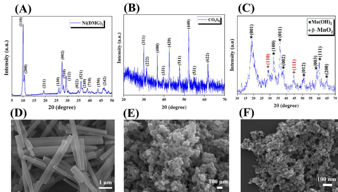
Fig. 4 Powder XRD of (A) Ni(DMG)<sub>2</sub> (B) Co<sub>9</sub>S<sub>8</sub> (C) Mn(OH)<sub>2</sub>. FE-SEM morphology (D) Ni(DMG)<sub>2</sub> (E) Co<sub>9</sub>S<sub>8</sub> (F) Mn(OH)<sub>2</sub>.
