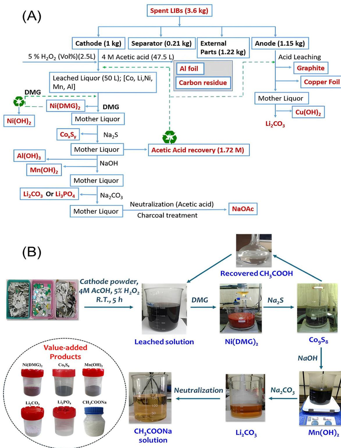
Fig. 8 (A) Flow sheet for a single batch of cathode and anode showing hydrometallurgical leaching & sequential chemical precipitation methods adopted in our studies using spent LIBs, and (B) digital images of the products recovered during the process.
