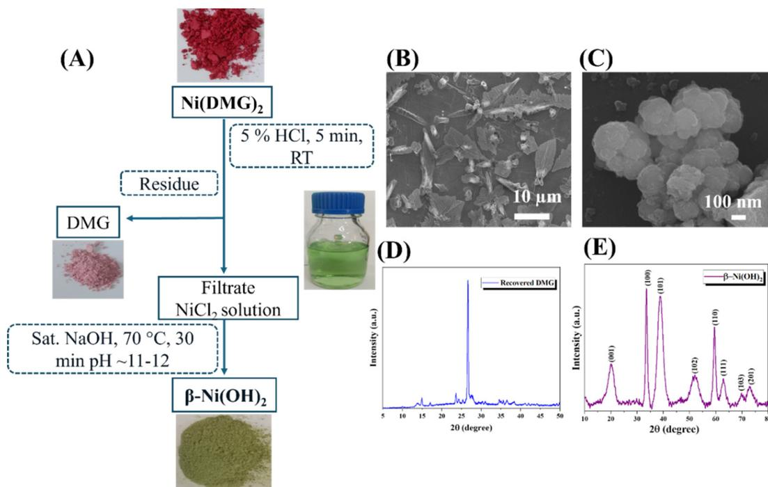
Fig. 6 (A) The flowchart for the recovery of Ni and DMG from the spent LIB-derived  $\text{Ni}(\text{DMG})_2$  complex. (B and C) FE-SEM morphology of recovered DMG and  $\beta\text{-Ni}(\text{OH})_2$ . (D and E) Powder XRD of recovered DMG and  $\beta\text{-Ni}(\text{OH})_2$ .
