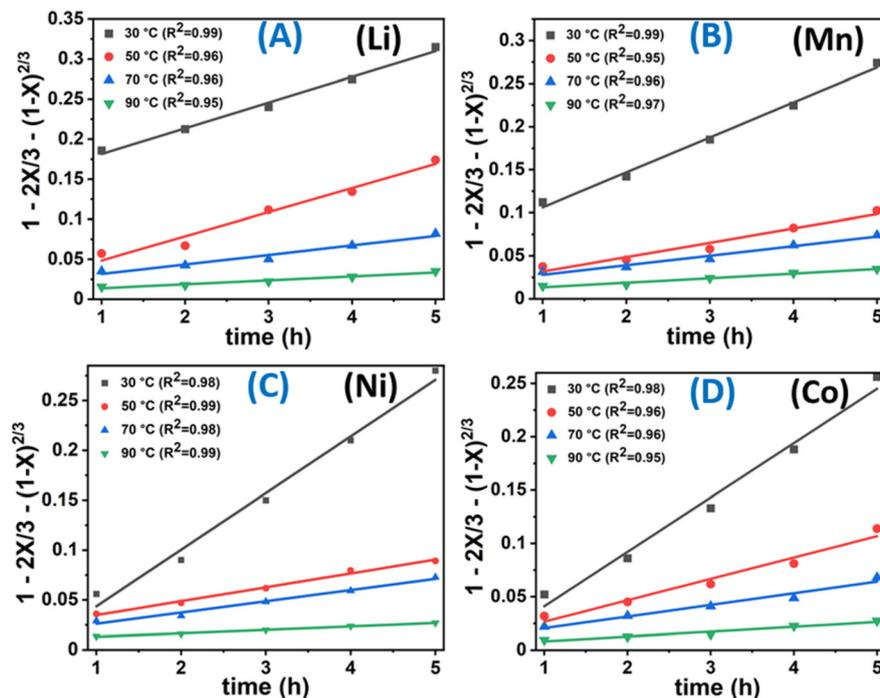
Fig. 3 (A) Plot between  $1 - 2X/3 - (1-X)^{2/3}$  versus time (h) for Li, (B) Mn, (C) Ni, and (D) Co under optimized conditions (S L<sup>-1</sup> ratio: 20 g L<sup>-1</sup>; H<sub>2</sub>O<sub>2</sub> conc: 5%; acetic acid conc: 4 M; time: 5 h) varying temperature.
