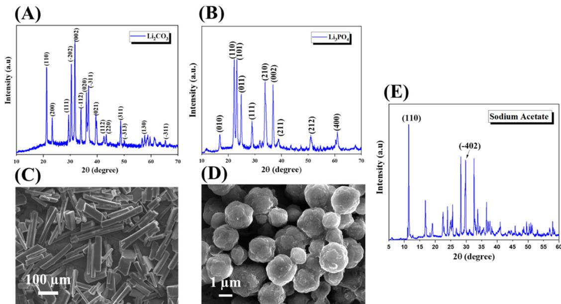
Fig. 5 (A and B) Powder XRD of recovered pure  $\text{Li}_2\text{CO}_3$  and  $\text{Li}_3\text{PO}_4$ . (C and D) FE-SEM morphology of  $\text{Li}_2\text{CO}_3$  and  $\text{Li}_3\text{PO}_4$ . (E) Powder XRD of crystalline sodium acetate.
