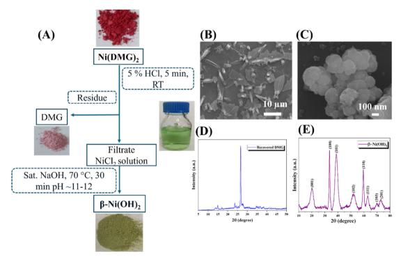
Fig. 6 (A) The flowchart for the recovery of Ni and DMG from the spent LIB-derived Ni(DMG)<sub>2</sub> complex. (B and C) FE-SEM morphology of recovered DMG and  $\beta$ -Ni(OH)<sub>2</sub>. (D and E) Powder XRD of recovered DMG and  $\beta$ -Ni(OH)<sub>2</sub>.
