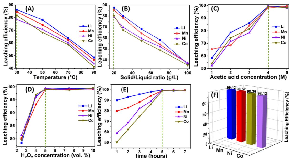
Fig. 2 The effects of (A) reaction temperature, (B) pulp density, (C) acid concentration, (D)  $\text{H}_2\text{O}_2$  dosage, (E) leaching time, and (F) leaching efficiencies of metals under optimized conditions.
