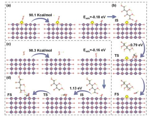
Fig. 5 (a) Dissociation energy of H<sub>2</sub>O<sub>2</sub> over the Ce<sub>1.0%</sub>-MgO catalyst and the adsorption energy of OOH. (b) Reaction energy barriers of glucose C1-C2 bond cleavage over the Ce<sub>1.0%</sub>-MgO catalyst. (c) Dissociation energy of H<sub>2</sub>O<sub>2</sub> over the MgO catalyst and the adsorption energy of OOH. (d) Reaction energy barriers of glucose C1-C2 bond cleavage over the MgO catalyst.
