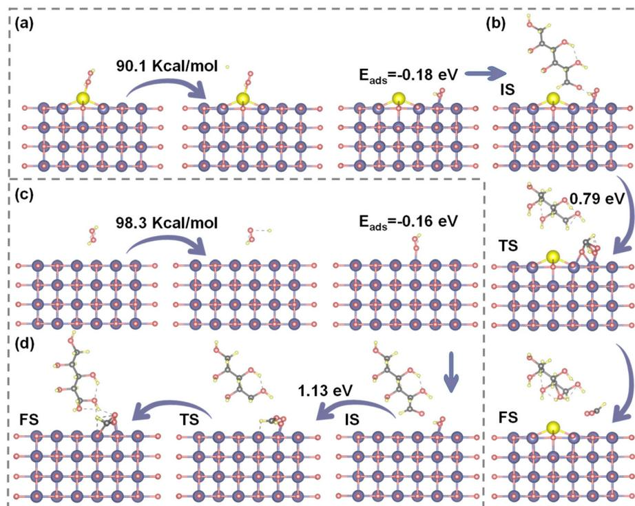
**Fig. 5** (a) Dissociation energy of  $\text{H}_2\text{O}_2$  over the  $\text{Ce}_{1.0\%}\text{-MgO}$  catalyst and the adsorption energy of  $\text{OOH}$ . (b) Reaction energy barriers of glucose C1-C2 bond cleavage over the  $\text{Ce}_{1.0\%}\text{-MgO}$  catalyst. (c) Dissociation energy of  $\text{H}_2\text{O}_2$  over the  $\text{MgO}$  catalyst and the adsorption energy of  $\text{OOH}$ . (d) Reaction energy barriers of glucose C1-C2 bond cleavage over the  $\text{MgO}$  catalyst.
