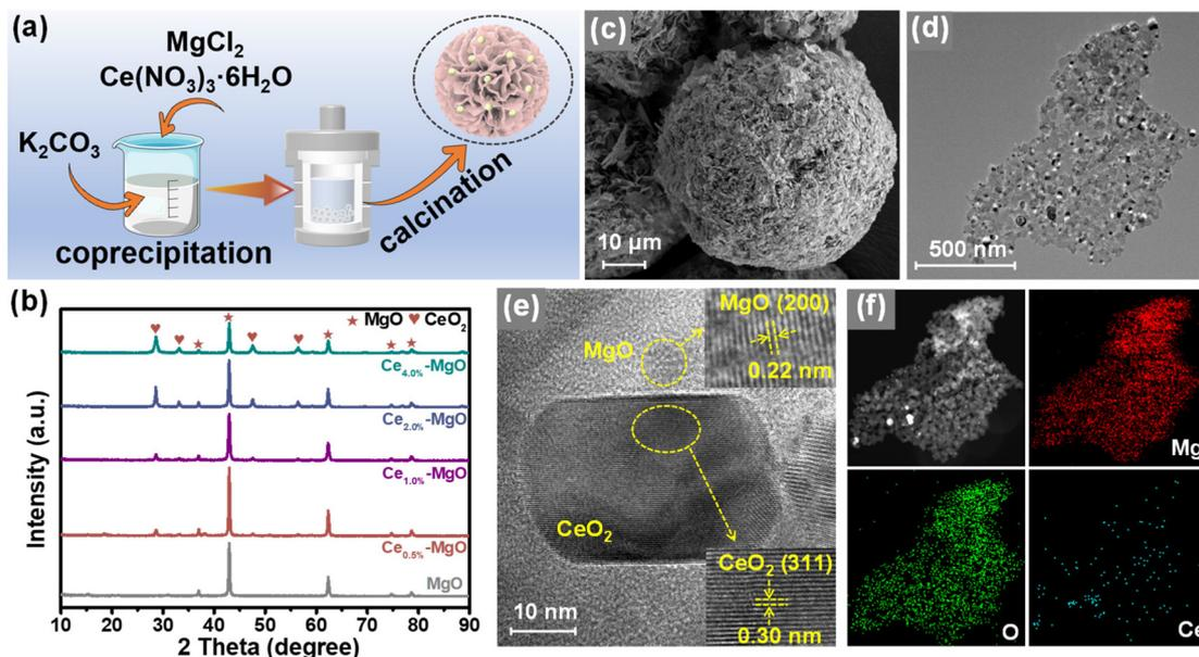
**Fig. 1** (a) Schematic illustration of the Ce–MgO catalyst synthesis process. (b) XRD patterns of the as-prepared MgO and Ce–MgO catalysts. (c) SEM, (d) TEM and (e) HRTEM images of the Ce<sub>1.0%</sub>–MgO catalyst and (f) corresponding elemental mapping.
