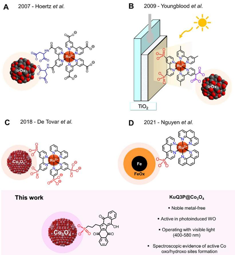
**Scheme 1** Photo(electro)catalytic dyadic systems for water oxidation (WO) based on transition metal oxide NPs functionalized with Ru-based molecular dyes (LHU) (top, A–D) and the **KuQ3P@Co<sub>3</sub>O<sub>4</sub>** hybrid nanomaterials presented in this work (bottom).
