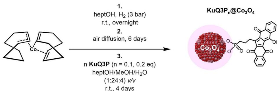
**Scheme 2** Synthesis of KuQ3P<sub>n</sub>@Co<sub>3</sub>O<sub>4</sub> dyads via (1) the organometallic approach, (2) controlled air oxidation of Co<sup>heptOH</sup> NPs and (3) Co<sub>3</sub>O<sub>4</sub><sup>heptOH</sup> NP sensitization with KuQ3P.
