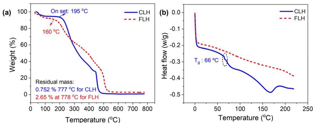
Fig. 5 (a) TGA isotherm, and (b) DSC isotherm of both cross-linked and functionalized hydrogel.
