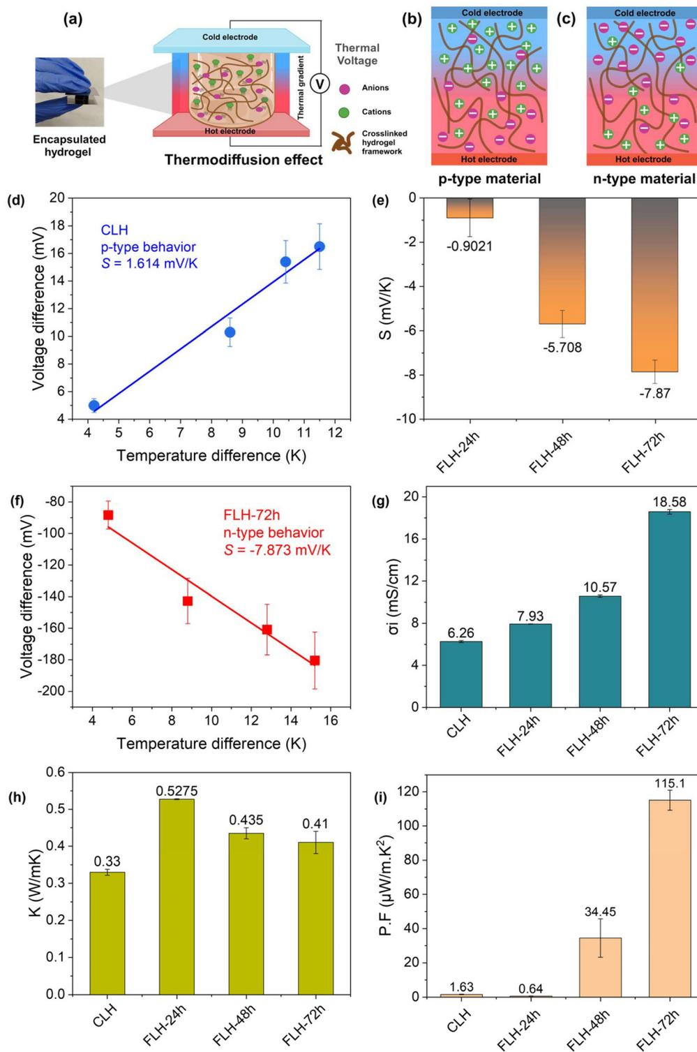
**Fig. 7** (a) Schematic representation of selective ion migration under thermidiffusion effect, (b) p-type material, (c) n-type material, (d) ionic Seebeck coefficient ( $S$ ) of CLH, (e) functionalized hydrogel under different time intervals, (f) ionic Seebeck coefficient of FLH-72 h, (g) ionic conductivity, (h) thermal conductivity and (i) power factor of hydrogel.
