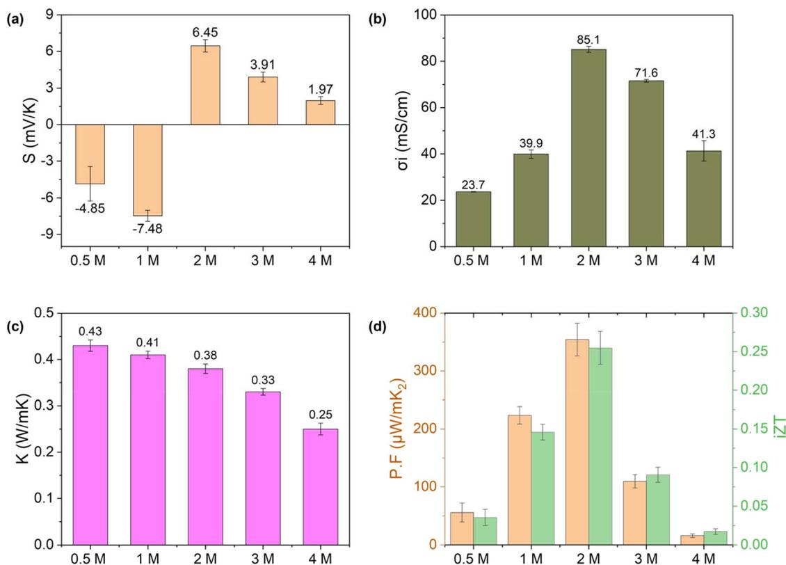
Fig. 9 Effect of electrolyte concentration in terms of (a) Seebeck coefficient, (b) ionic conductivity, (c) thermal conductivity, and (d) power factor and figure of merit of functionalized hydrogel FLH-72 h.
