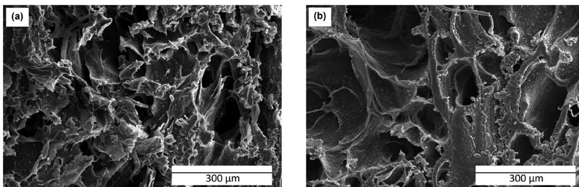
Fig. 4 SEM images of (a) the cross-linked and (b) functionalized hydrogel.
