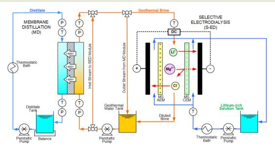
Fig. 1 Schematic representation of the conceptual lab-scale integration of DCMD and S-ED for simultaneous water and Li recovery from geothermal brine.
