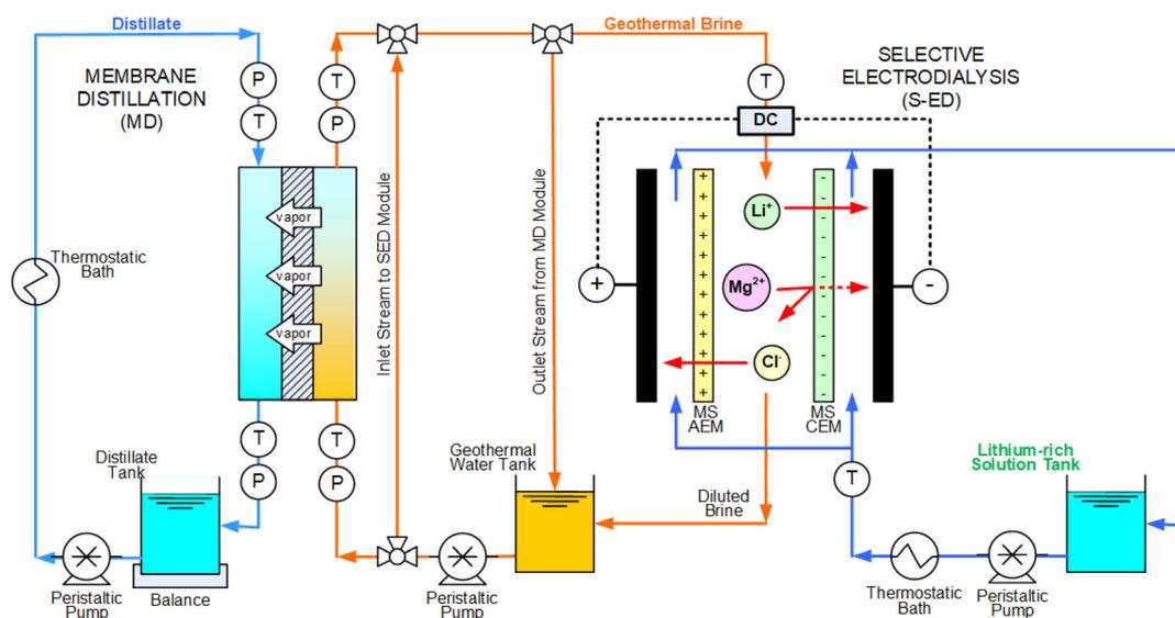
**Fig. 1** Schematic representation of the conceptual lab-scale integration of DCMD and S-ED for simultaneous water and Li recovery from geothermal brine.
