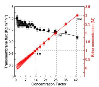
**Fig. 2** DCMD treatment of geothermal water: the variation of transmembrane flux *versus* and brine (feed) concentration vs concentration factor.
