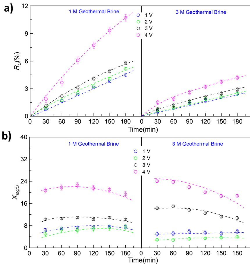
Fig. 4 Effect of applied voltage on (a) recovery rate of Li<sup>+</sup> at 1 M and 3 M; (b) Mg/Li ratio of concentrate stream vs. duration of time at 1 M and 3 M.
