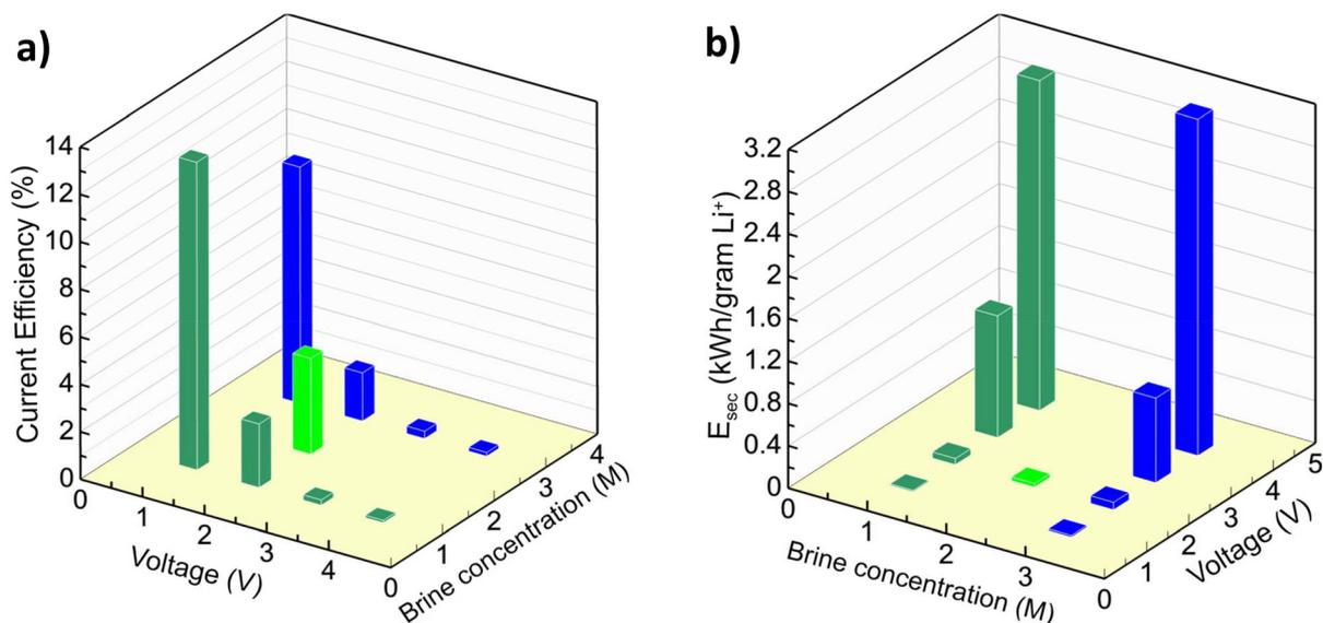
**Fig. 8** (a) Average current efficiency at varying voltages for 1 M and 3 M concentrations, and at different concentrations (1 M, 2 M, and 3 M) at a constant voltage of 2 V. (b) Average specific energy consumption at varying voltages for 1 M and 3 M concentrations, and at different concentrations (1 M, 2 M, and 3 M) at a constant voltage of 2 V.
