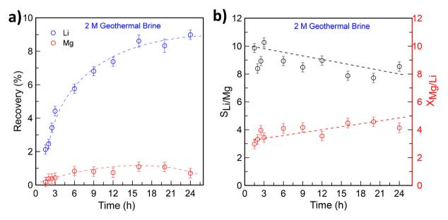
Fig. 9 Long-term performance evaluation of S-ED, showing (a) the recovery rates of Li<sup>+</sup> and Mg<sup>2+</sup> and (b) the selectivity and Mg/Li ratio in the concentrate stream over 24 h. Experiments were conducted with a 2 M geothermal brine feed under an applied voltage of 2 V to assess membrane stability and separation efficiency.
