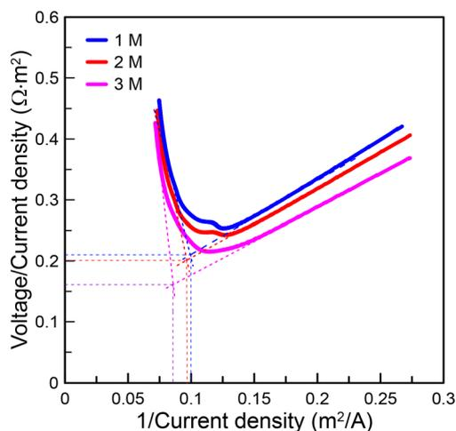
Fig. 3 LCD determination by Cowan and Brown method.
