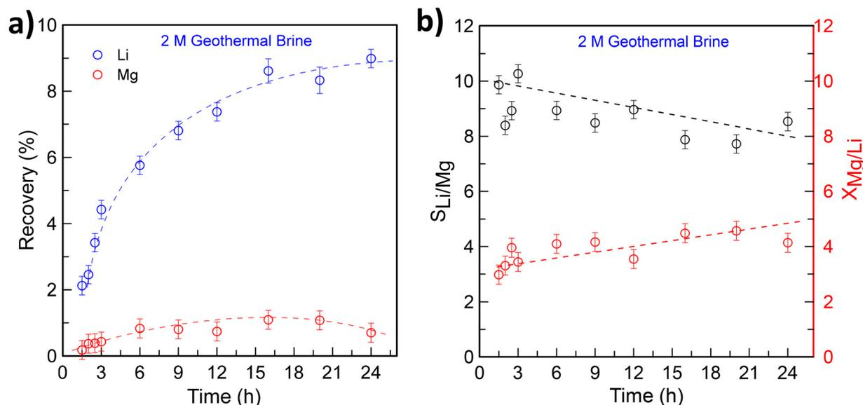
**Fig. 9** Long-term performance evaluation of S-ED, showing (a) the recovery rates of  $\text{Li}^+$  and  $\text{Mg}^{2+}$  and (b) the selectivity and  $\text{Mg/Li}$  ratio in the concentrate stream over 24 h. Experiments were conducted with a 2 M geothermal brine feed under an applied voltage of 2 V to assess membrane stability and separation efficiency.
