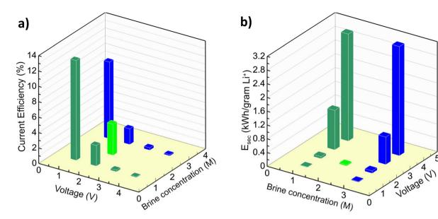
Fig. 8 (a) Average current efficiency at varying voltages for 1 M and 3 M concentrations, and at different concentrations (1 M, 2 M, and 3 M) at a constant voltage of 2 V. (b) Average specific energy consumption at varying voltages for 1 M and 3 M concentrations, and at different concentrations (1 M, 2 M, and 3 M) at a constant voltage of 2 V.
