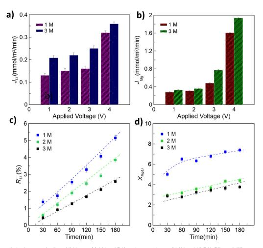
Fig. 6 Effect of applied voltage on the flux of lithium at (a) 1 M and 3 M, and magnesium at (b) 1M and (d) 3 M. Effect of different concentrations on (c) recovery rate of Li<sup>+</sup> and (d) Mg/Li ratio of concentrate stream. The applied voltage remains at 2 V in all cases.
