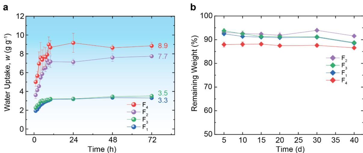
**Fig. 3** Water uptake and stability of the biobased self-blown PC foams over time. (a) Maximum ( $w = 8.9 \text{ g g}^{-1}$ ) and minimum ( $w = 3.3 \text{ g g}^{-1}$ ) water uptake within 72 h, depending on the polyols used. (b) *In vitro* degradation behavior of the foams in neutral pH water for 40 days.
