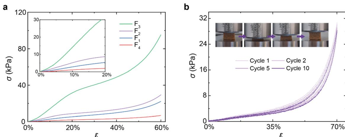
**Fig. 4** Mechanical properties via compression testing of the biobased self-blown PC foams. (a) Stress–strain ( $\sigma$ – $\epsilon$ ) curves of foams F<sub>1</sub>–F<sub>4</sub> with different biobased polyols. (b)  $\sigma$ – $\epsilon$  curves of the CNSL-based foam, F<sub>2</sub>, for 10 compression and release cycles up to 70% strain. Inset: photographs of F<sub>2</sub> being subjected to cyclic compression.
