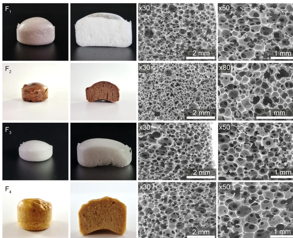
**Fig. 2** Pictures and SEM characterization of the biobased self-blown PC foams presented in Table 1.
