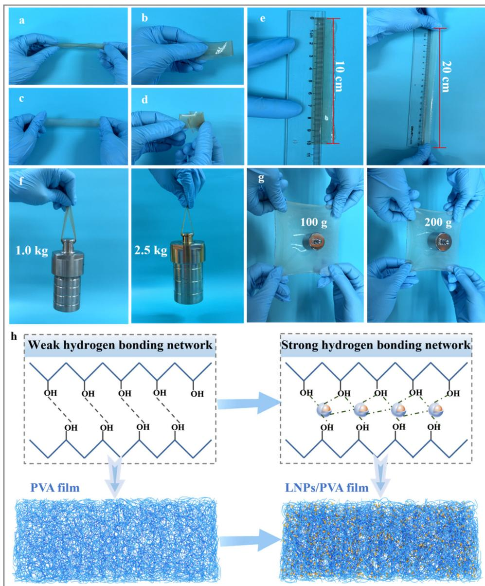
**Fig. 8** Demonstration of the superior mechanical properties of LNP/PVA composite films. (a) Curling; (b) bending; (c) stretching; (d) folding; (e) elongation to twice the original length; (f) withstanding tension; (g) withstanding pressure; (h) interweaving diagram of LNPs and PVA.
