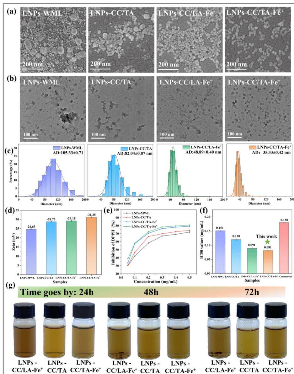
Fig. 6 Chemical characteristics analysis of LNPs. (a) SEM; (b) TEM; (c) grain size distribution map; (d) zeta potential; (e) DPPH free radical scavenging; (f)  $IC_{50}$  values; (g) water dispersion stability.
