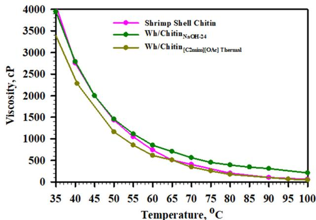
Fig. 4 Viscosity measurements for 2.5 wt%  $[C_2mim][OAc]$  solutions of shrimp shell chitin extracted with  $[C_2mim][OAc]$  (pink), mushroom chitin pulped with NaOH for 24 h (dark green), and mushroom chitin extracted with  $[C_2mim][OAc]$ -thermal (olive).
