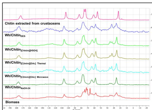
Fig. 3 Comparison of solid-state <sup>13</sup>C multiCP-MAS NMR spectra of biomass (red) and isolated materials from (olive) pulping with NaOH-24 h, (green) extraction with [C<sub>2</sub>mim][OAc]-microwave, (cyan) extraction with [C<sub>2</sub>mim][OAc]-thermal, (blue) pulping with [C<sub>4</sub>mim][HSO<sub>4</sub>], (purple) pulping with 2 : 1 lactic acid : [Cho]Cl, (pink) chitin extracted from crustacean biomass using [C<sub>2</sub>mim][OAc].
