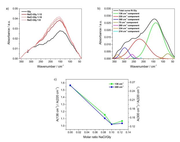
Fig. 3 (a) Experimental FIR spectra of pure Gly and Gly-based mixtures. (b) Deconvolution bands (c)  $A(300 \text{ cm}^{-1})/A(220 \text{ cm}^{-1})$  and  $A(136 \text{ cm}^{-1})/A(220 \text{ cm}^{-1})$  as a function of the molar ratio.
