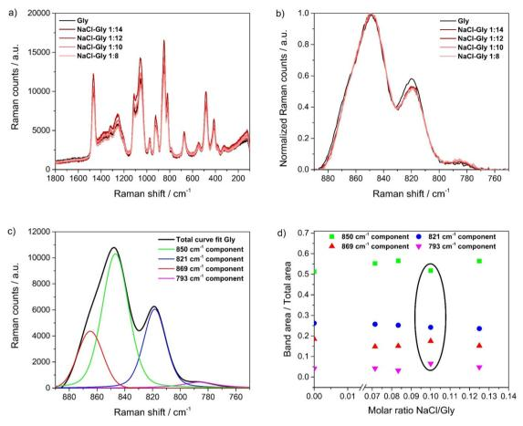
Fig. 2 (a) Experimental Raman spectra of pure Gly and Gly-based mixtures. (b) Normalized Raman spectra in the region 750–890 cm<sup>-1</sup>. (c) Deconvolution bands. (d) Trend of the component areas as a function of concentration.
