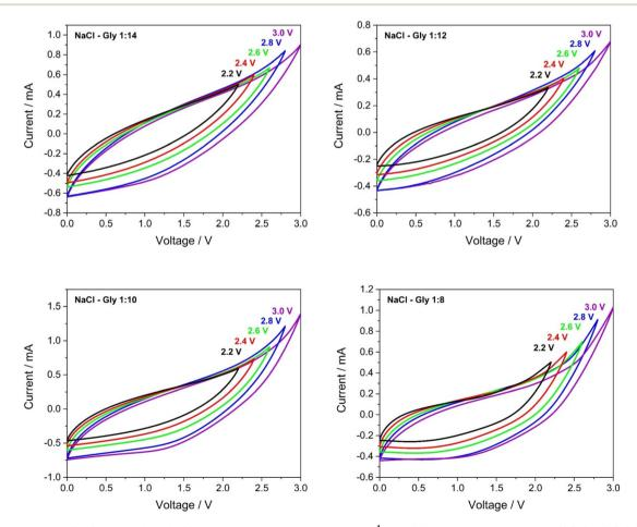
Fig. 6 CV curves of NaCl-Gly electrolytes in AC supercapacitors acquired at 1 mV s<sup>-1</sup> with different operational voltages (2.2, 2.4, 2.6, 2.8, 3 V).
