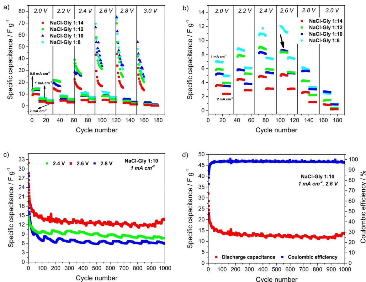
**Fig. 7** (a) Specific capacitance vs. cycle number for NaCl-Gly electrolytes obtained with 10 cycles GCD at different cut-off voltages (2.2, 2.4, 2.6, 2.8, and 3 V) and current densities (0.5, 1 and 2  $\text{mA cm}^{-2}$ ). (b) Magnified view of (a) showing cycling at 1 and 2  $\text{mA cm}^{-2}$ . (c) Comparison between specific capacitance of NaCl-Gly 1 : 10 at 2.4, 2.6, and 2.8 V. (d) Specific capacitance and coulombic efficiency vs. cycle number of NaCl-Gly 1 : 10 at 2.6 V.
