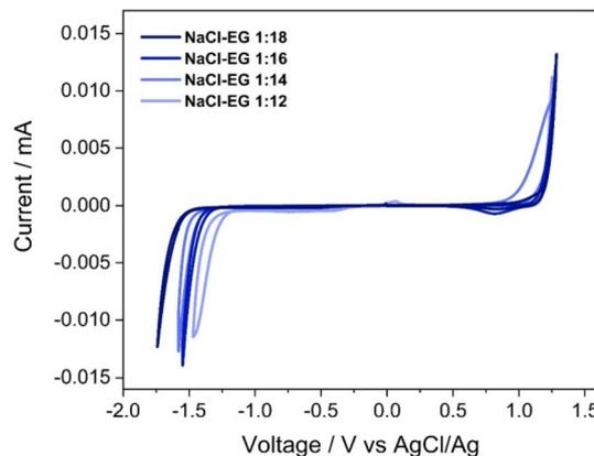
**Fig. 5** ESW of NaCl-polyols electrolytes by using carbon as the working electrode at 1 mV s<sup>-1</sup>.
