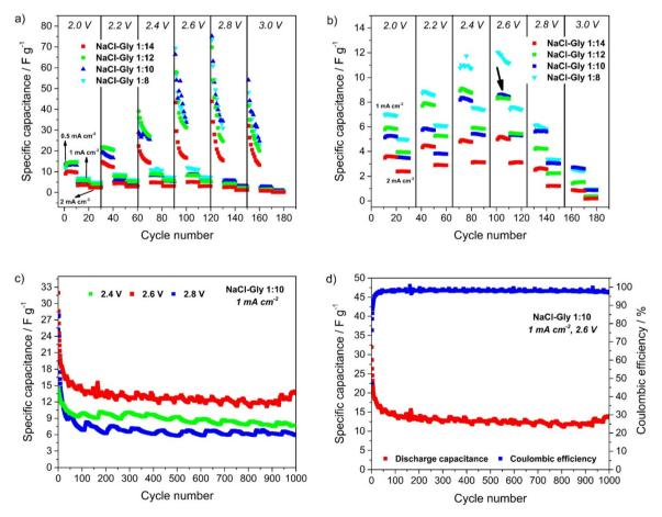
Fig. 7 (a) Specific capacitance vs cycle number for NaCl-Gly electrolytes obtained with 10 cycles GCD at different cut-off voltages (2.2, 2.4, 2.6, 2.8, and 3 V) and current densities (0.5, 1 and 2 mA cm<sup>-2</sup>). (b) Magnified view of (a) showing cycling at 1 and 2 mA cm<sup>-2</sup>. (c) Comparison between specific capacitance of NaCl-Gly 1:10 at 2.4, 2.6, and 2.8 V. (d) Specific capacitance and coulombic efficiency vs cycle number of NaCl-Gly 1:10 at 2.6 V.
