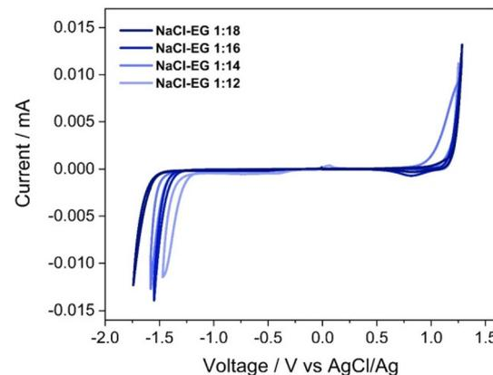
**Fig. 5** ESW of NaCl-polyols electrolytes by using carbon as the working electrode at 1 mV s<sup>-1</sup>.
