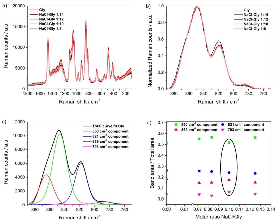
**Fig. 2** (a) Experimental Raman spectra of pure Gly and Gly-based mixtures. (b) Normalized Raman spectra in the region 750–890  $\text{cm}^{-1}$ . (c) Deconvolution bands. (d) Trend of the component areas as a function of concentration.
