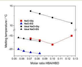
**Fig. 1** Melting temperatures vs molar ratio HBA/HBD of NaCl–Gly and NaCl–EG mixtures and ideal behaviour ruled by cryoscopic depression calculated according to the equation  $\Delta T = i \times K_{\rm cr} \times {\rm molality} \ (K_{\rm cr,Gly} = 3.56~{\rm ^{\circ}C} \ {\rm Kg \ mol^{-1}}, \ K_{\rm cr,EG} = 3.11~{\rm ^{\circ}C} \ {\rm Kg \ mol^{-1}}).$
