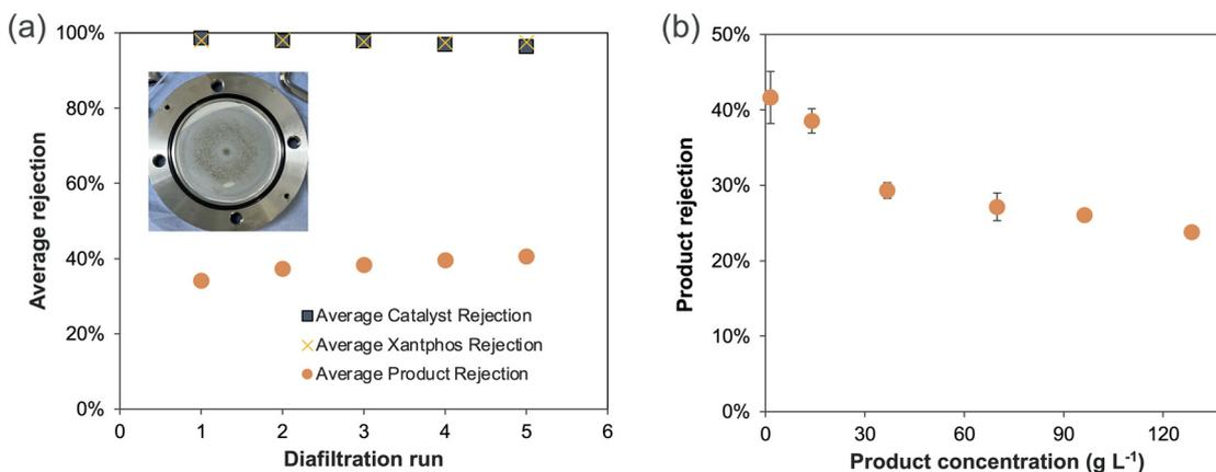
**Fig. 7** (a) The average catalyst and product rejection in each diafiltration cycle. Inset: photo of the Borsig oNF-1 membrane coupon after five cycles of catalyst reuse experiments. (b) The rejection of Stage 2 product at varying product concentrations. The feed solution was prepared by diluting the Stage 2 reaction mixture with 2-MeTHF to the desired concentration.
