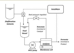
Fig. 2 Flowchart of the Minimem cross-flow system with an AutoMem system for diafiltration.
