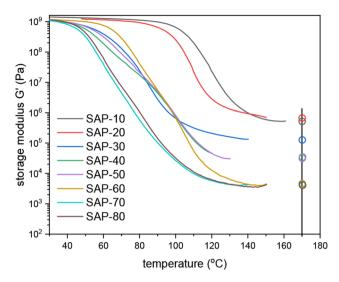
Fig. 5 Storage modulus of extracted SAP-10 to SAP-80 *versus* temperature. Note: 170 °C (vertical black line) was chosen as the point where  $G_x$  was taken; since all curves reached a plateau before 150 °C it is reasonable to predict the G' value according to the existing curve. The circles are the predicted point at 150 °C.
