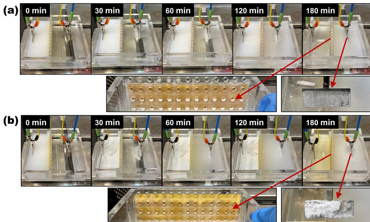
**Fig. 4** Time-lapse images of the cement clinker precursor electrolyzer showing the precipitation process of  $\text{Ca}(\text{OH})_2$  during electrolysis and the precipitation behavior of the  $\text{Ca}(\text{OH})_2$  product on the membrane and electrode after 3 h of electrolysis at various  $\text{Ca}^{2+}$  concentrations in the catholyte. (a) Without  $\text{Ca}^{2+}$  and (b) with 0.2 M  $\text{Ca}^{2+}$  in the initial catholyte.
