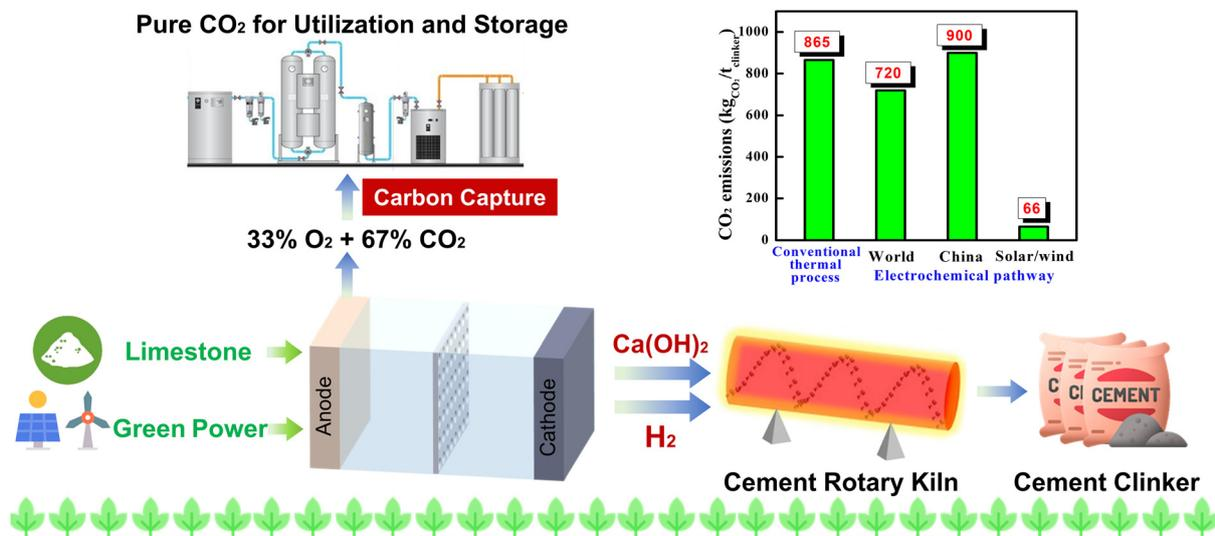
**Fig. 1** A scheme of the electrochemical-based, low-carbon emission cement clinker production process. The carbon emissions during this process only come from electricity consumption, which can be reduced by over 90% at a cell voltage of 2.5 V and a current efficiency of 90% if using green electricity. Grid emission factors: world = 0.43 kg CO<sub>2</sub> per kW per h, China = 0.54 kg CO<sub>2</sub> per kW per h, solar or wind energy = 0.04 kg CO<sub>2</sub> per kW per h.<sup>2,13,15–17</sup>
