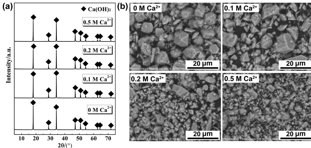
Fig. 5 (a) XRD patterns and (b) SEM images of the precipitation products collected from the cathode chamber, membrane and electrode after electrolysis at various  $\text{Ca}^{2+}$  concentrations in the initial catholyte.
