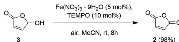
Fig. 4 TEMPO-mediated aerobic oxidation from HFO to MA (Feringa *et al.*, 2022).<sup>27</sup>
