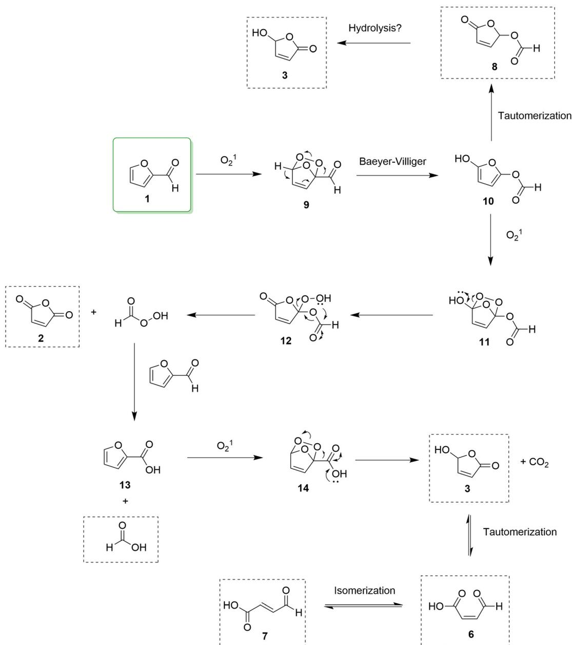
Fig. 3 Plausible pathway for the  $\text{O}_2^1$  oxidation of furfural towards various reaction products.
