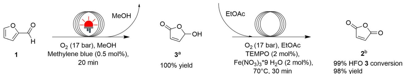
Fig. 6 Continuous flow oxidation of FUR 1 to MA 2 without intermediate purification. <sup>a</sup> Yield is determined *via* quantitative HPLC analysis after first reaction step. <sup>b</sup> Yield and conversion are determined *via* <sup>1</sup>H-NMR analysis with mesitylene as internal standard which was added after the first reaction step.
