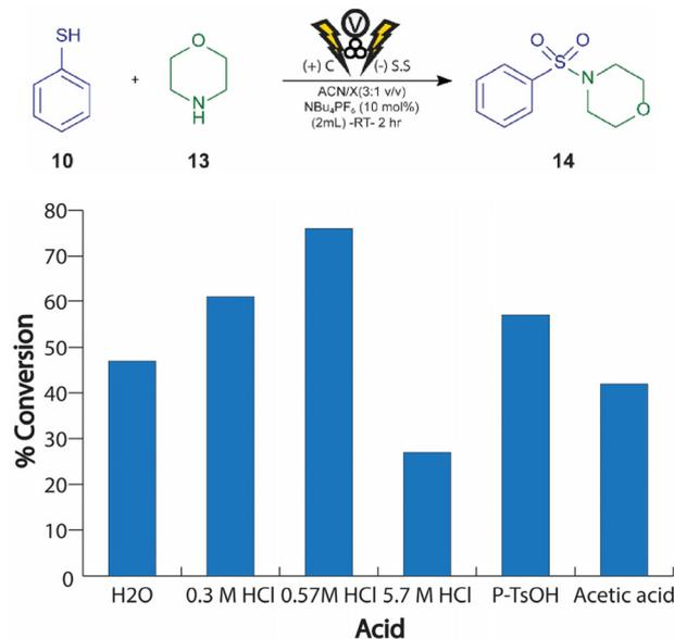
Fig. 5 Optimizing the conditions for mechano-electrochemical oxidative coupling of thiols and amines (1 mmol scale reaction, 110 mg of **10**,  $\eta = 8.3 \mu\text{L mg}^{-1}$ , voltage applied =  $-3.4 \text{ V}$ ).
