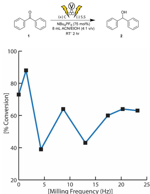
**Fig. 3** Screening the impact of milling frequency on the mechanochemically mediated-electrochemical reduction of benzophenone using MEC-1. (0.9 mmol scale, 160 mg of **1**), 90 mol% TBAPF<sub>6</sub>,  $\eta = 50 \mu\text{L mg}^{-1}$ .  $V = -4.5 \text{ V}$ .
