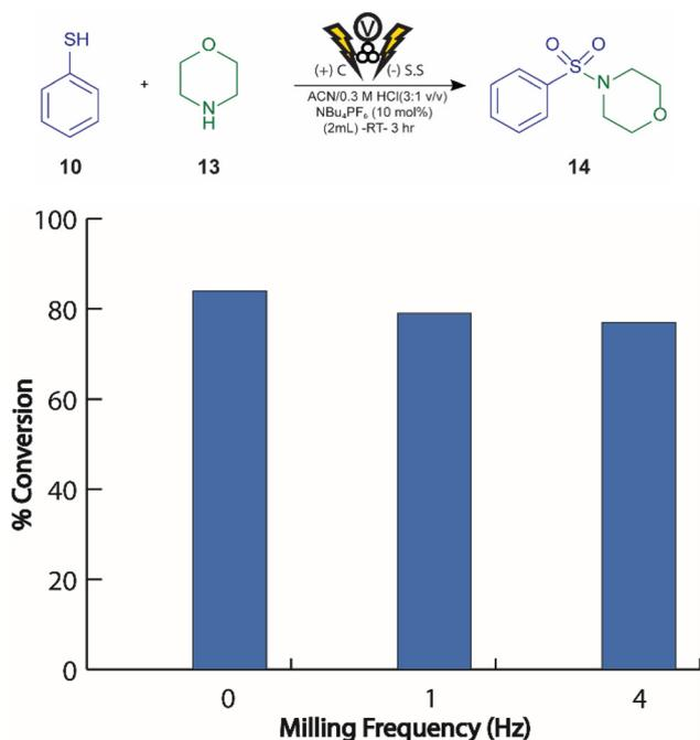
Fig. 4 Screening the impact of milling frequency on the electrochemical oxidative coupling of thiophenol and morpholine (1 mmol scale reaction, 110 mg of **10**,  $\eta = 8.3 \mu\text{L mg}^{-1}$ , voltage applied =  $-3.4 \text{ V}$ ).
