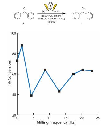
Fig. 3 Screening the impact of milling frequency on the mechanochemically mediated-electrochemical reduction of benzophenone using MEC-1. (0.9 mmol scale, 160 mg of 1), 90 mol% TBAPF6,  $\eta$  = 50  $\mu$ L mg<sup>-1</sup>. V = -4.5 V
