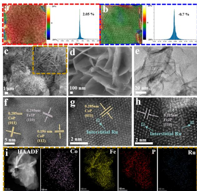
**Fig. 1** (a and b) GPA (geometric phase analysis) test of FeCoP/FF-Q and FeCoP/FF-C electrodes. (c and d) SEM images of Ru-FeCoP/FF. (e) TEM image of powders on the surface of the Ru-FeCoP/FF electrode. (f) HRTEM images of powders on the surface of the Ru-FeCoP/FF electrode. (g and h) HAADF-STEM images of powders on the surface of the Ru-FeCoP/FF electrode. (i) EDX elemental mappings of powders on the surface of the Ru-FeCoP/FF electrode.
