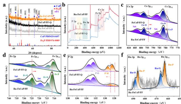
**Fig. 2** (a) XRD patterns of Ru-FeCoP/FF, FeCoP/FF-Q and Ru-FeCoP/FF-C electrodes. (b) XPS surveys of Ru-FeCoP/FF and FeCoP/FF-Q electrodes. High-resolution spectra of (c) Co 2p, (d) Fe 2p, (e) P 2p, (f) Ru 3p of Ru-FeCoP/FF and FeCoP/FF-Q electrodes.
