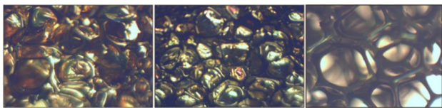
Fig. 10 Optical microscopy photographs showing the morphologies of humins foams as a function of reaction temperatures (from left to right 220, 230 and 400 °C). 95
