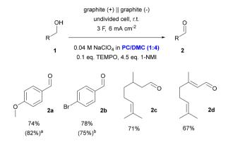
**Scheme 1** Preparative-scale TEMPO-mediated oxidation of different alcohols. Yields determined with  $^1\mathrm{H}$  NMR spectroscopy using mesitylene as an internal standard.  $^a$  0.2 M NaClO<sub>4</sub>.  $^b$  Isolated yield.
