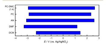
Fig. 1 Electrochemical windows of PC and a PC/DMC mixture (1:4, w/w) compared to common solvents used in organic electrosynthesis. Determined using cyclic voltammetry at v=10 mV s<sup>-1</sup> using a glassy carbon working electrode (threshold current density: 0.1 mA cm<sup>-2</sup>). Supporting electrolyte: 0.1 M Bu<sub>4</sub>NBF<sub>4</sub>.;<sup>1</sup>
