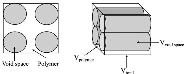
**Fig. 7** Representative diagram of the internal structure of a foam. By determining the  $V_{\text{polymer}}$ ,  $V_{\text{void space}}$ , and  $V_{\text{total}}$ , the porosity of a foam can be calculated.
