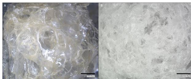
**Fig. 8** Optical microscope images of the cross-section of (A) P(DEAEMS<sub>70-co</sub>-MVPA<sub>30</sub>) and (B) EPS foam peanuts at 20 times magnification.
