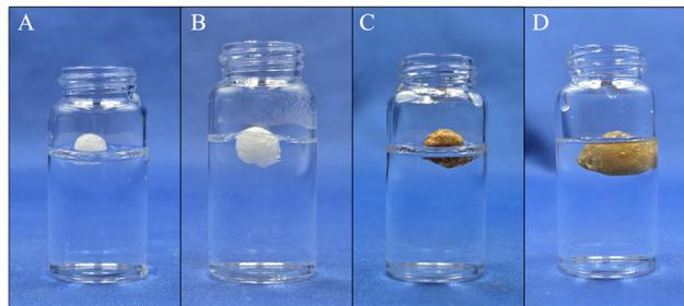
**Fig. 15** Water resistance test comparison between virgin P(DEAEMS<sub>70-co</sub>-MVPA<sub>30</sub>) and recycled P(DEAEMS<sub>70-co</sub>-MVPA<sub>30</sub>) in neutral water. (A) Virgin P(DEAEMS<sub>70-co</sub>-MVPA<sub>30</sub>) at time = 0. (B) Virgin P(DEAEMS<sub>70-co</sub>-MVPA<sub>30</sub>) after 5 days. (C) Recycled P(DEAEMS<sub>70-co</sub>-MVPA<sub>30</sub>) at time = 0. (D) Recycled P(DEAEMS<sub>70-co</sub>-MVPA<sub>30</sub>) after 5 days.
