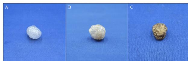
**Fig. 13** Colour change of P(DEAEMS<sub>70</sub>-co-MVPA<sub>30</sub>) foam after recycling cycles. (A) Pristine foam, no recycling performed. (B) P(DEAEMS<sub>70</sub>-co-MVPA<sub>30</sub>) foam after two recycling cycles. (C) P(DEAEMS<sub>70</sub>-co-MVPA<sub>30</sub>) foam after five recycling cycles.
