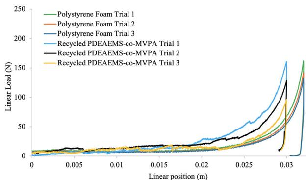
**Fig. 16** Force deflection curves for P(DEAEMS<sub>70-co</sub>-MVPA<sub>30</sub>) and EPS foam peanuts. Samples were mounted into an Instron 8521 equipped with a 5 kN transducer load cell and crushed at a rate 0.1 mm s<sup>-1</sup>. The compression strength was determined by using the measured force at 50% the  $L_0$  (approximately 0.02 m) divided by the  $A_0$  of the sample.
