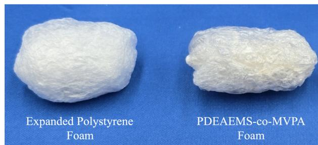
Fig. 6 Image of EPS foam peanut and P(DEAEMS<sub>70-co</sub>-MVPA<sub>30</sub>) foam.
