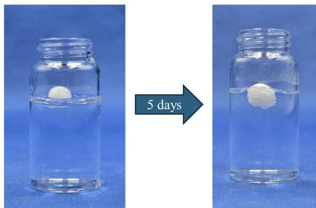
**Fig. 9** Water resistance test of P(DEAEMS<sub>70-co</sub>-MVPA<sub>30</sub>) foam in neutral water. Over 5 days there was no observed disintegration or damage to the foam.
