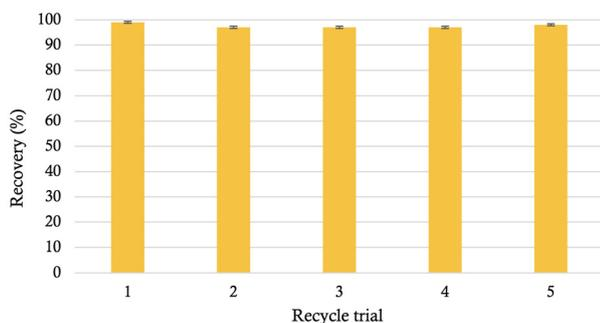
**Fig. 12** Percent recovery of P(DEAEMS<sub>70</sub>-co-MVPA<sub>30</sub>) over different recycling cycles. Percent recovery was determined by analyzing the final mass of polymer compared to the start mass of the polymer for each trial. Average recovery was determined to be  $\geq 98\%$ .
