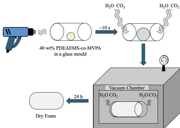
Fig. 5 Preparation method of P(DEAEMS<sub>70-co</sub>-MVPA<sub>30</sub>) foam.
