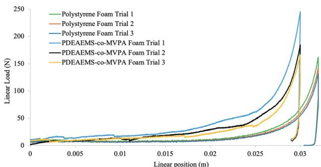
**Fig. 10** Force deflection curves for P(DEAEMS<sub>70-co-MVPA</sub><sub>30</sub>) and EPS foam peanuts. Samples were mounted into an Instron 8521 equipped with a 5 kN transducer load cell and crushed at a rate  $0.1 \text{ mm s}^{-1}$ . The compression strength was determined by using the measured force at 50% the  $L_0$  (approximately 0.02 m) divided by the  $A_0$  of the sample.
