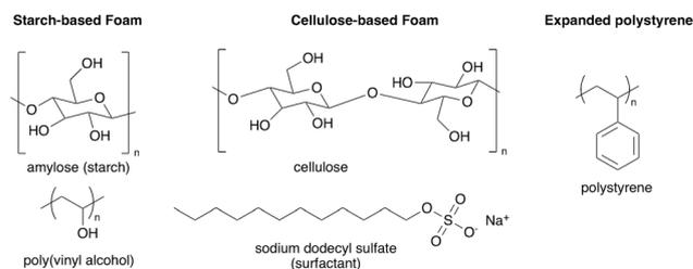
**Fig. 1** Components in biobased and petroleum-based foams. (Left) Starch-based foam is comprised of starch and the polymeric stabilizer polyvinyl alcohol. (Center) Cellulose-based foam contains cellulose and a surfactant (SDS given as an example). (Right) Expanded polystyrene only contains polystyrene.
