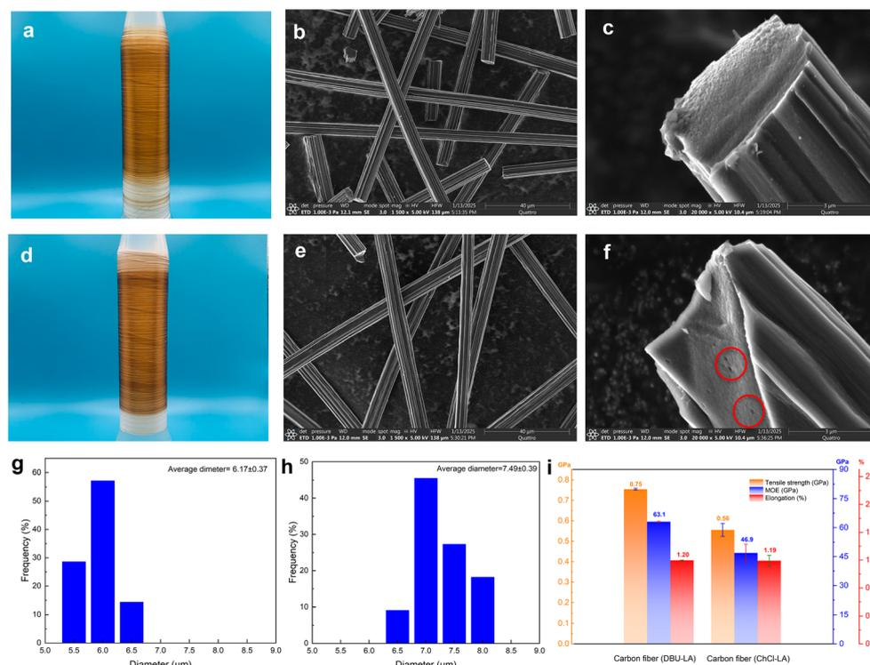
**Fig. 5** Morphology and mechanical properties of lignin-based carbon fiber. (a, b and c) Photograph and SEM image of DBU-LA pretreated lignin carbon fiber; (d, e and f) photograph and SEM image of ChCl-LA pretreated lignin carbon fiber; (g and h) diameter of the DBU-LA pretreated lignin and ChCl-LA pretreated lignin carbon fiber; (i) mechanical performance of lignin-based carbon fiber.
