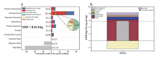
Fig. 3 TEA and LCA results of bio-catechol production in the baseline scenario. (a) Breakdown of MSP. (b) Breakdown of GWP with that of fossilderived catechol indicated by the dashed line
