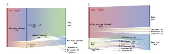
Fig. 2 (a) Mass balance of feedstock (kg  $h^{-1}$ ) and (b) energy balance (MJ  $h^{-1}$ ) of the conceptual biorefinery (baseline scenario).
