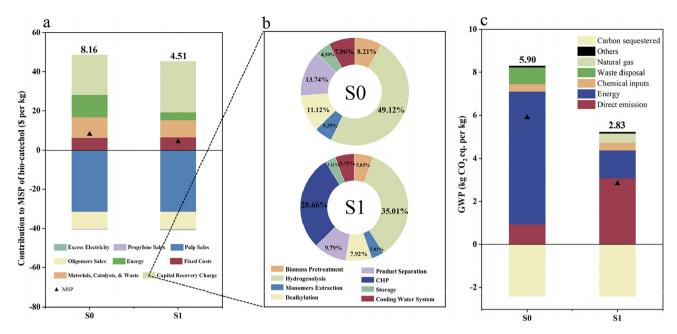
Fig. 4 TEA and LCA results of bio-catechol production in S0 and S1. (a) Breakdown of MSP. (b) Breakdown of total capital recovery charge based on different processes. (c) Breakdown of GWP based on types of inputs.
