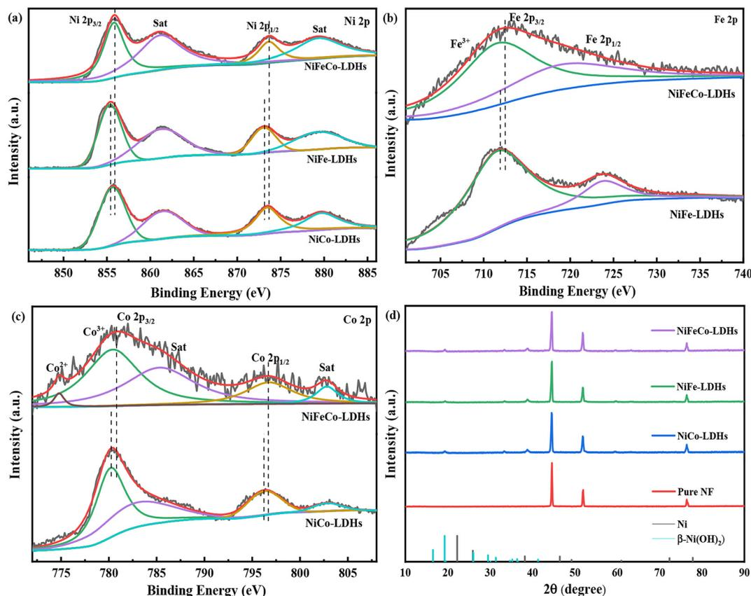
Fig. 2 XPS spectra of NiFeCo-LDHs: (a) Ni 2p, (b) Fe 2p and (c) Co 2p. (d) XRD patterns of NiFeCo-LDHs, NiFe-LDHs, NiCo-LDHs, and pure NF.
