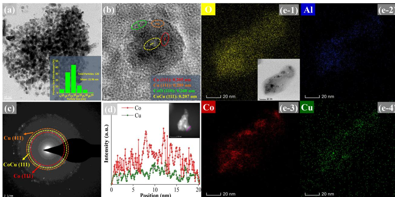
Fig. 1 TEM (a), HR-TEM (b), SAED (c), HAADF-STEM line scan (d), and mapping (e1–4) of the reduced Co<sub>5</sub>CuAl catalyst.
