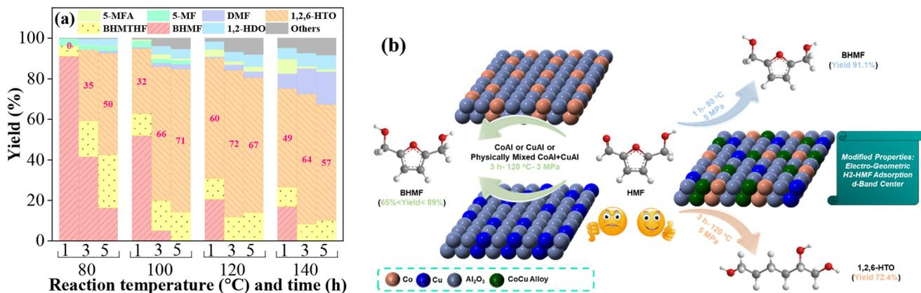
Fig. 5 (a) Effects of time/temperature on HMF hydrogenation/hydrogenolysis. Reaction conditions: 30 mg Co<sub>5</sub>CuAl, 10 mL methanol, 1 mmol HMF, 5 MPa. (b) Schematic diagram of the catalytic hydrogenation/hydrogenolysis of HMF into BHMF and/or 1,2,6-HTO.
