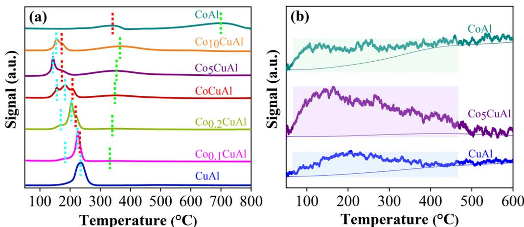
Fig. 2 (a) H<sub>2</sub>-TPR and (b) H<sub>2</sub>-TPD patterns of various LDOs.
