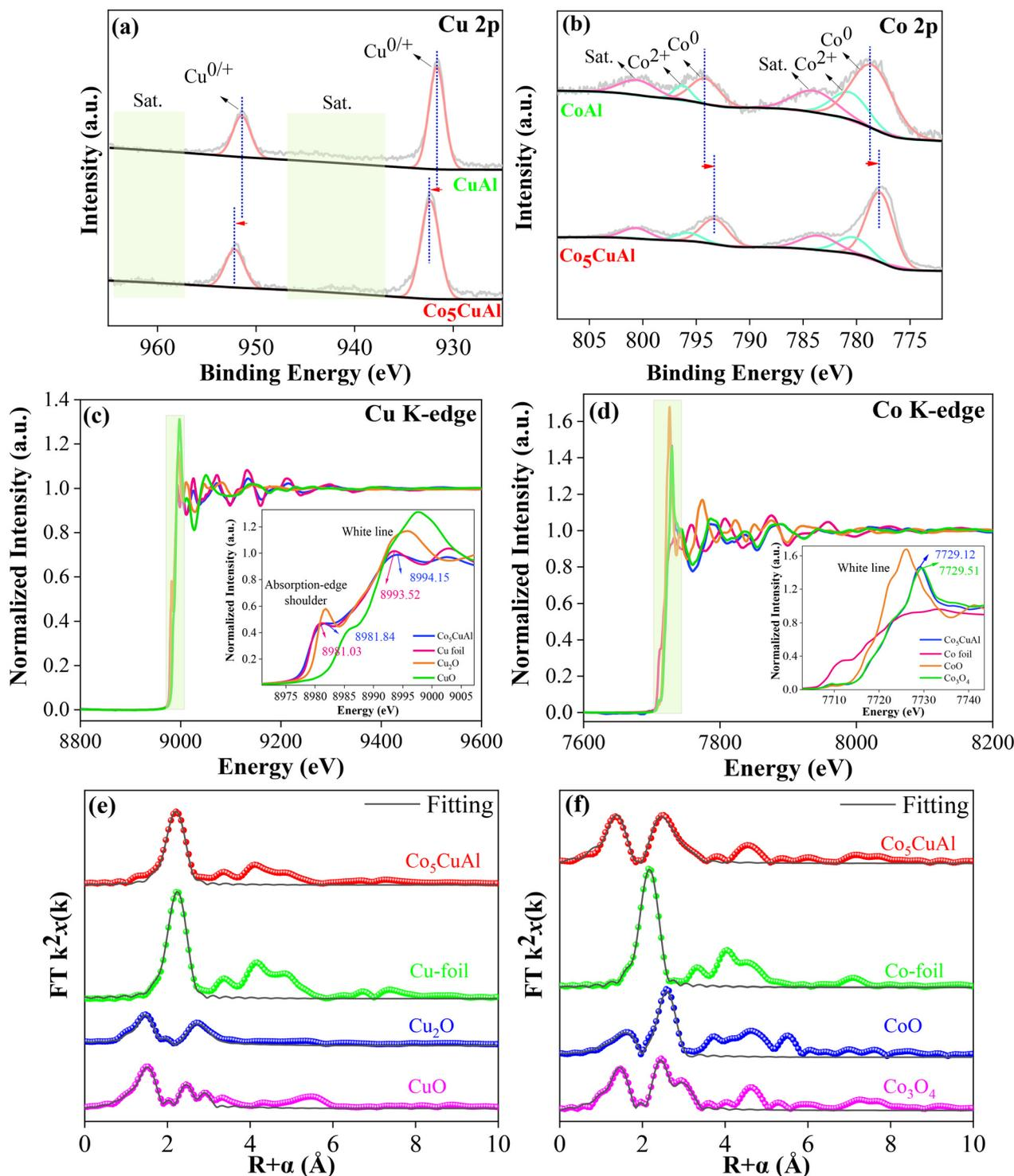
**Fig. 3** *In situ* XPS spectra of (a) Cu 2p and (b) Co 2p for the CuAl, CoAl, and Co<sub>5</sub>CuAl catalysts. Cu and Co K-edge XANES (c and d) and EXAFS spectra (e and f) of the Co<sub>5</sub>CuAl catalyst and standard samples.
