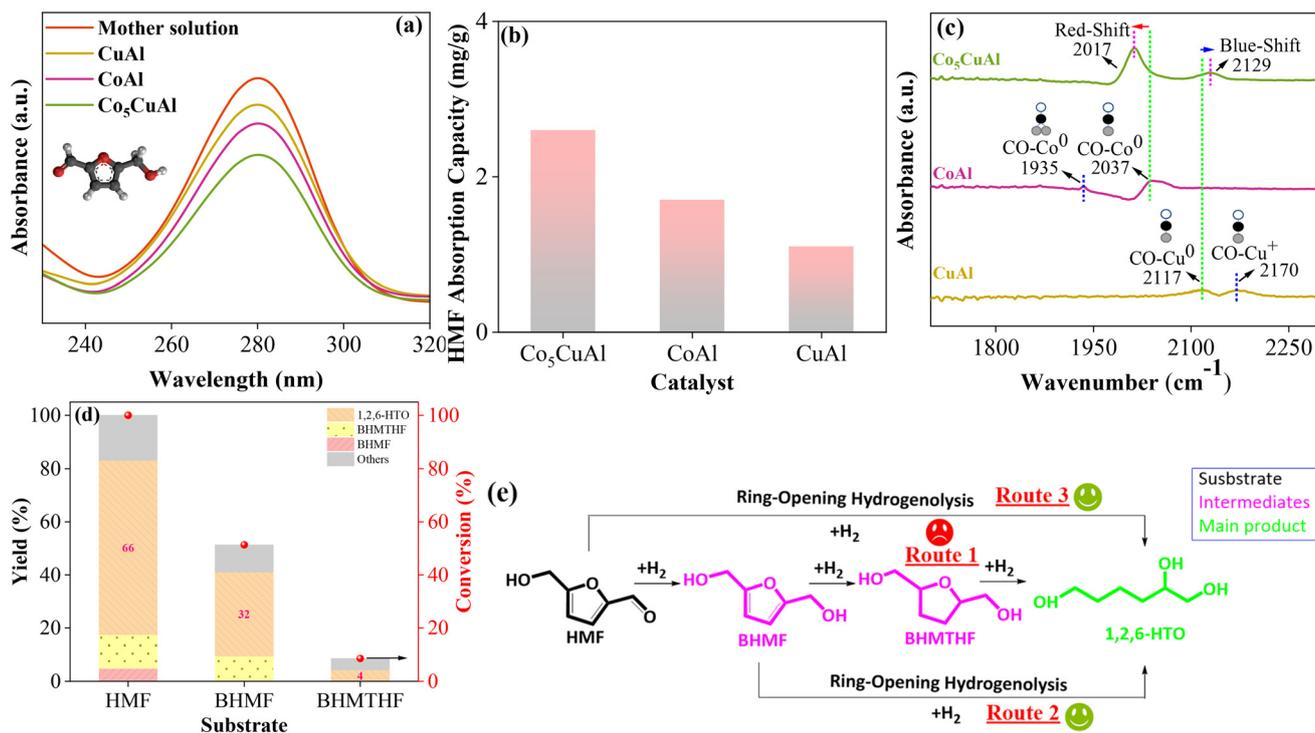
**Fig. 6** (a) UV-vis spectra of the residual solutions after HMF adsorption, (b) HMF adsorption capacity, and (c) CO-FTIR after flushing with Ar for 5 min at 30 °C. (d) Hydrogenation/hydrogenolysis of HMF, BHMf, and BHMTHF over Co<sub>5</sub>CuAl. Reaction conditions: 30 mg Co<sub>5</sub>CuAl, 10 mL methanol, 1 mmol substrate, 2 h, 120 °C, 5 MPa. (e) A plausible reaction pathway for HMF transformation into 1,2,6-HTO over Co<sub>5</sub>CuAl.
