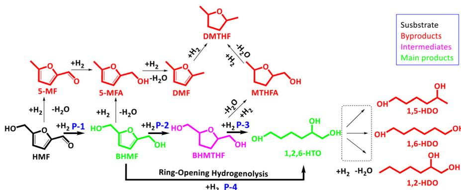
**Scheme 1** The reaction pathways for HMF conversion into BHMF and 1,2,6-HTO.
