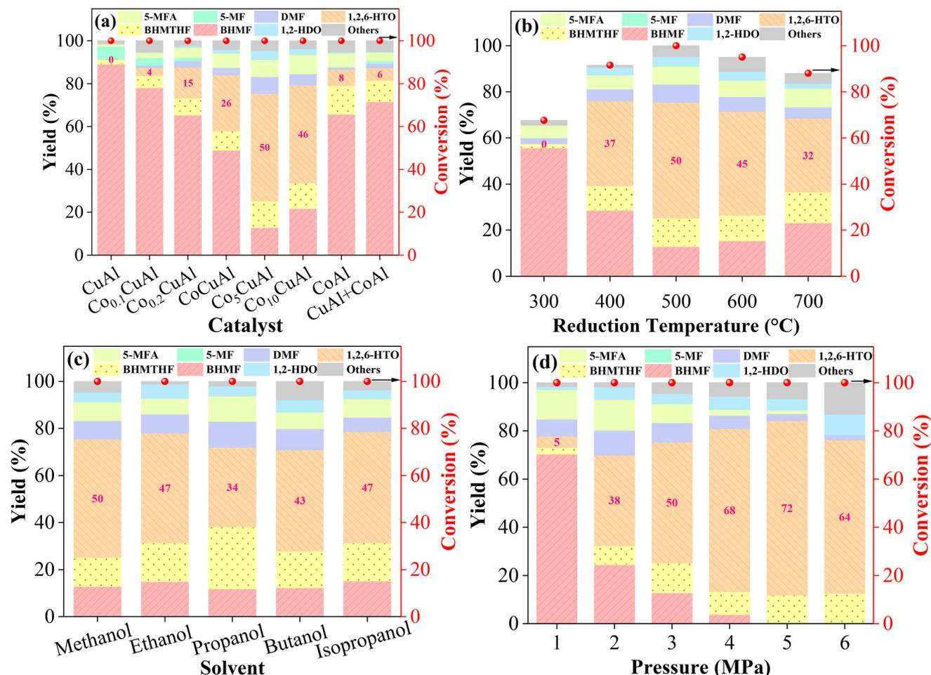
**Fig. 4** Effects of the (a) LDO composite and (b) Co<sub>5</sub>CuAl reduction temperature on HMF hydrogenation/hydrogenolysis. Reaction conditions: 30 mg catalyst, 10 mL methanol, 1 mmol HMF, 120 °C, 3 h, 3 MPa H<sub>2</sub>. Effects of (c) solvent and (d) H<sub>2</sub> pressure on HMF hydrogenation/hydrogenolysis. Reaction conditions: 30 mg Co<sub>5</sub>CuAl, 10 mL solvent, 1 mmol HMF, 120 °C, 3 h ((c) 3 MPa H<sub>2</sub>, (d) methanol).
