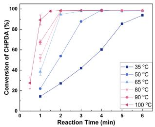
Fig. 8 Effect of reaction temperature on the reaction rate. Reaction conditions: n(TBACI): n(CHPDA): n(NaOH) = 0.05:1:1.8. The concentrations of TBACI and NaOH solutions are 20 wt%.
