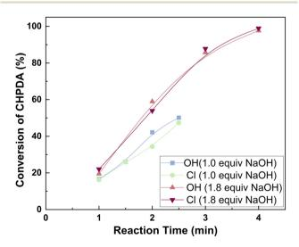
**Fig. 6** Effect of anions in PTCs on the dehydrochlorination rate. Reaction conditions: n(TBAX): n(CHPDA): n(NaOH) = 0.05:1:1.8 and T = 50 °C. Both the catalyst and NaOH are added in the form of 20 wt% solutions.
