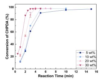
Fig. 7 Effect of alkali concentrations on the dehydrochlorination rate. Reaction conditions: n(TBACI): n(CHPDA): n(NaOH) = 0.05:1:1.8 and T=50 °C. The concentrations of the TBACI and NaOH solutions are 20 wt%.
