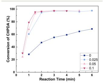
Fig. 9 Effect of n(TBACl)/n(CHPDA) on the reaction. Reaction conditions: n(NaOH): n(CHPDA) = 1.05: 1 and T = 100 °C, and the concentrations of the TBACl and NaOH solutions are 20 wt%.
