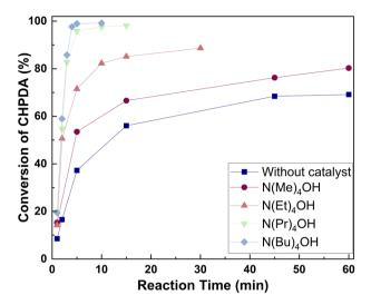
Fig. 5 Effect of PTC cations on the dehydrochlorination rate. Reaction conditions: n(catalyst): n(CHPDA): n(NaOH) = 0.05:1:1.8 and T = 50 °C. Both the catalyst and NaOH are added in the form of 20 wt% solutions. TMAOH = tetramethylammonium hydroxide, TEAOH = tetraethylammonium hydroxide, TPAOH = tetrapropylammonium hydroxide, and TBAOH = tetrabutylammonium hydroxide.
