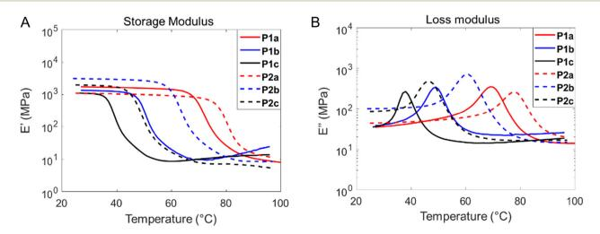
Fig. 4 DMA temperature sweep showing the (A) storage moduli, E', and (B) loss moluli, E'' of the obtained polyesters.
