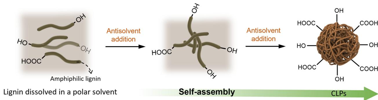
Fig. 4 A schematic proposal for the formation of CLPs by self-assembly.
