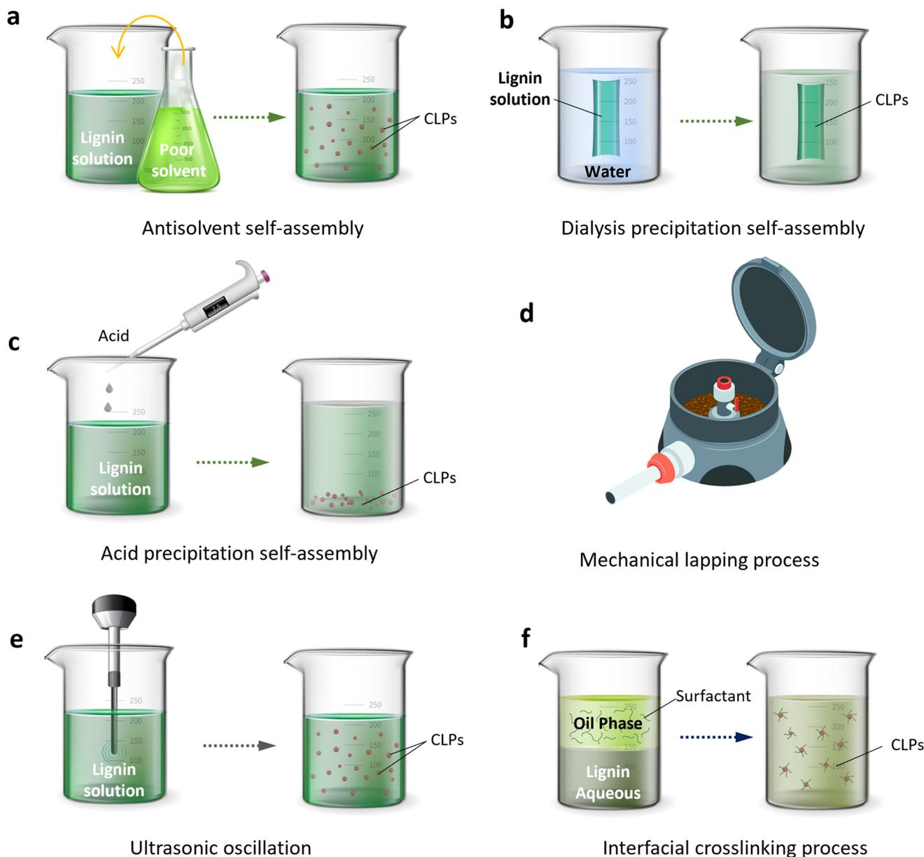
**Fig. 3** Preparation methods of CLPs. Antisolvent self-assembly of CLPs (a); dialysis precipitation self-assembly of CLPs (b); acid precipitation self-assembly of CLPs (c); mechanical lapping process of CLPs (d); ultrasonic oscillation of CLPs (e); interfacial crosslinking process of CLPs (f).
