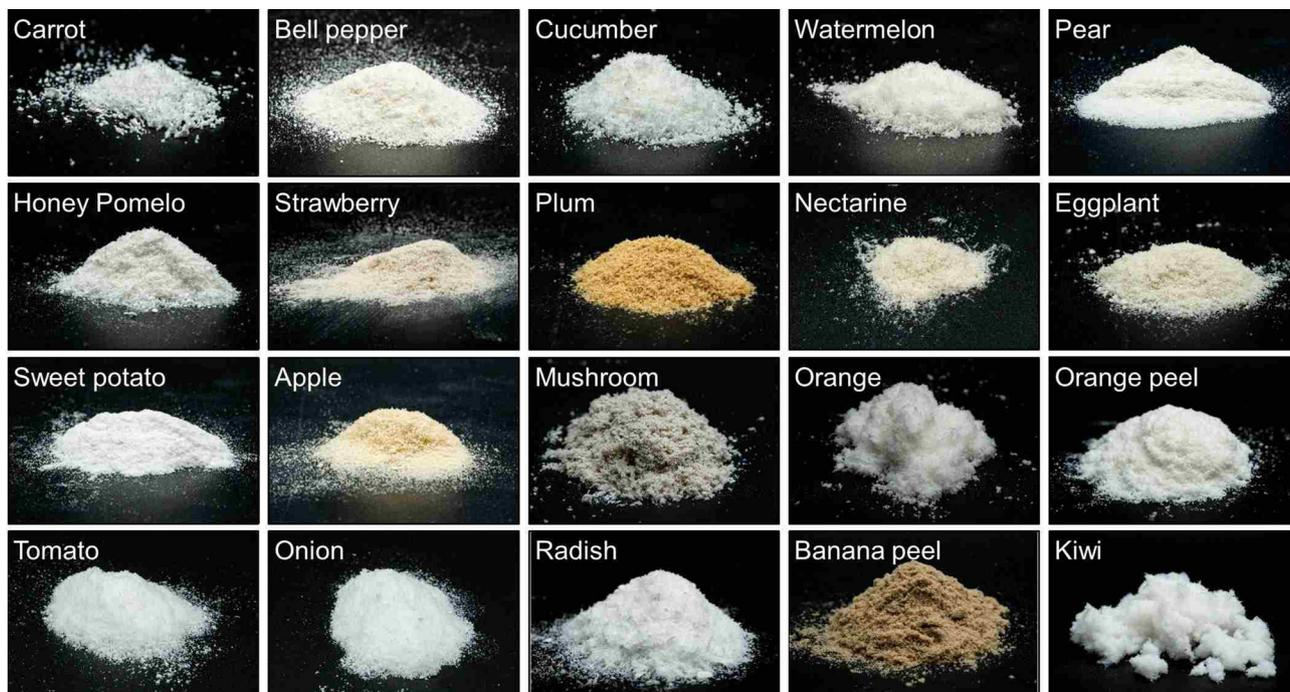
Fig. 2 Images of powders obtained after solvent exchange and sCO<sub>2</sub>-drying of various natural tissues. Respective sample names are given in the individual images.
