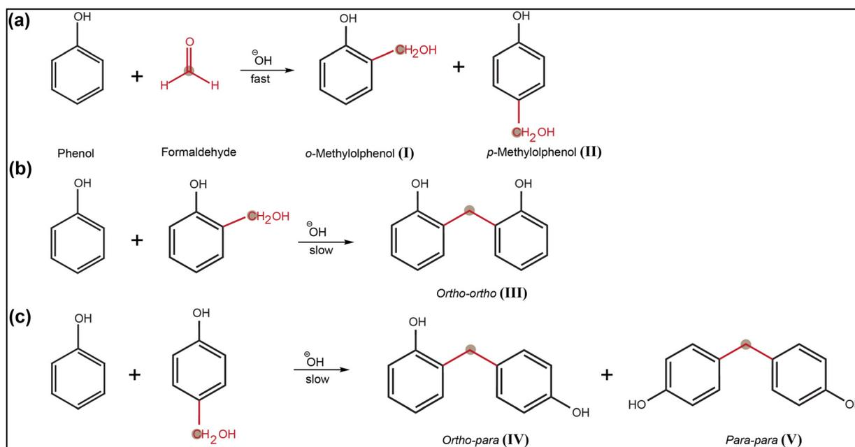
**Fig. 3** Reaction of phenol with formaldehyde. (a) *ortho* and *para*-methylphenols formation (I and II), (b) *ortho-ortho* methylene linkage formation (III), (c) *ortho-para* and *para-para* methylene linkage formation (IV and V). Here, linkages coming from formaldehyde are represented in red color, and labeled carbons are brown circles.
