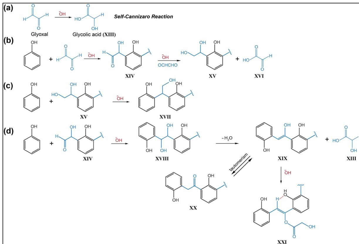
**Fig. 11** Reaction of phenol and glyoxal. (a) Self-Cannizzaro reaction of glyoxal forms glycolic acid (XI); (b) *ortho* substitution of phenol forms  $-\text{CH}(\text{OH})-\text{CHO}$  (XII) and  $-\text{CH}(\text{OH})-\text{CH}_2\text{OH}$  (XIII). Also oxidized form of glyoxal (XIV); (c) formation of dibenzyl derivative with  $\text{CHCH}_2\text{OH}$  (XV); (d) formation of compound XVIII and compound XIX (enol ester). Compound XIX is stabilized by hydrogen bonding.
