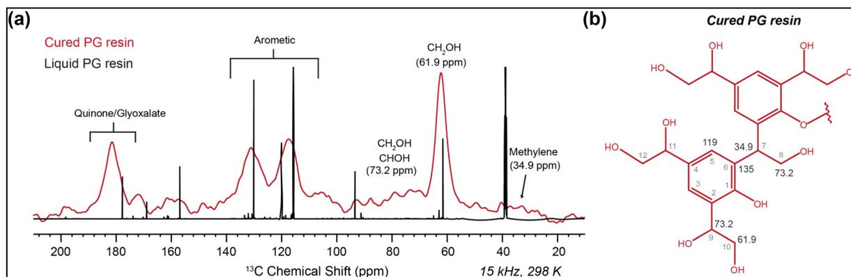
**Fig. 12** (a) Comparison of liquid  $^{13}\text{C}$  NMR spectra of liquid PG resin with the  $^{13}\text{C}$ -CP MAS spectra of cured PG resin ( $\text{CH}_2\text{OH}$  at 61.9 ppm and methylene linkage at 34.9 ppm) (b) dimer fragment of the polymeric cured PG resin consists of both  $\text{CH}_2\text{OH}$  group and methylene linkage.
