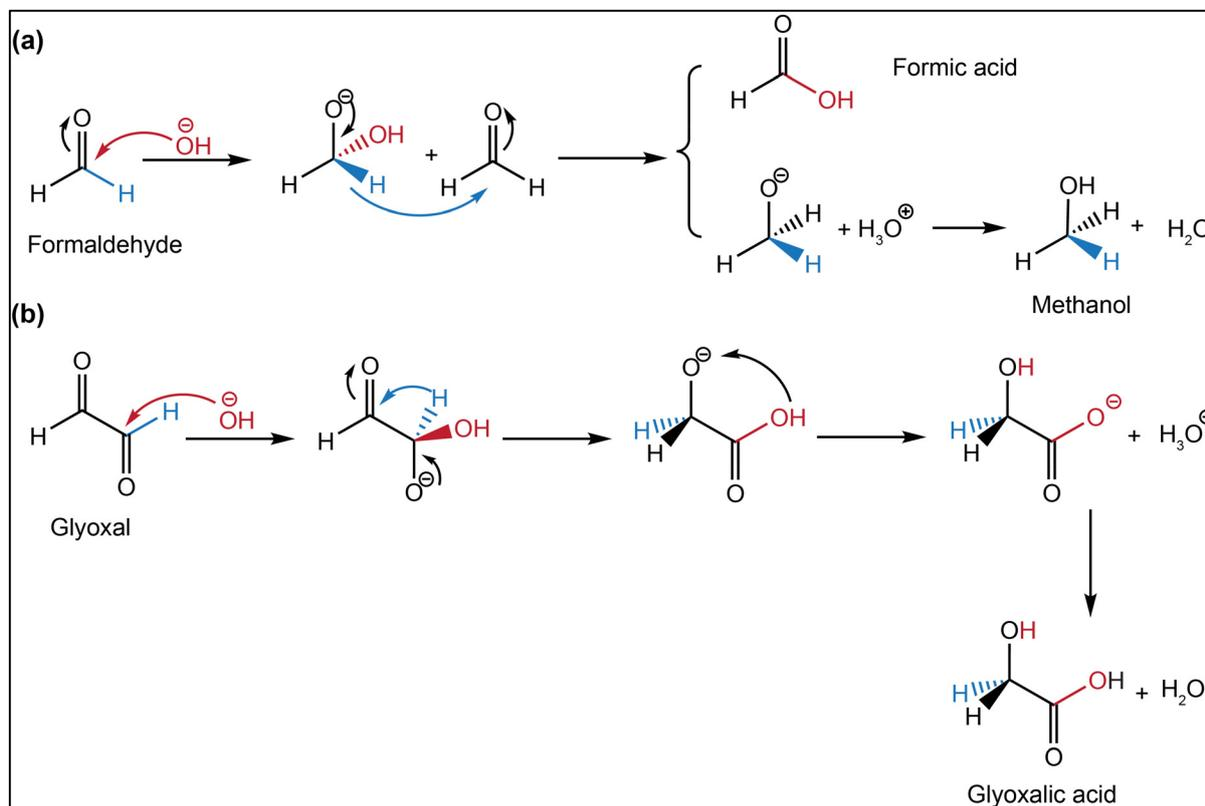
Fig. 2 Proposed mechanism of the self-Cannizzaro reaction of (a) Formaldehyde, (b) Glyoxal.<sup>16</sup>
