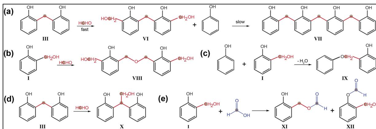
Fig. 4 Different condensation reactions of PF resin. (a) Formation of tetramer (VII) from dimer (III); (b) formation of dibenzyl ether through two  $\text{CH}_2\text{OH}$  (VIII); (c) formation of phenyl benzyl ether (IX); (d) reaction of methylene linkage with formaldehyde forms compound X; (e) formation of formate esters.
