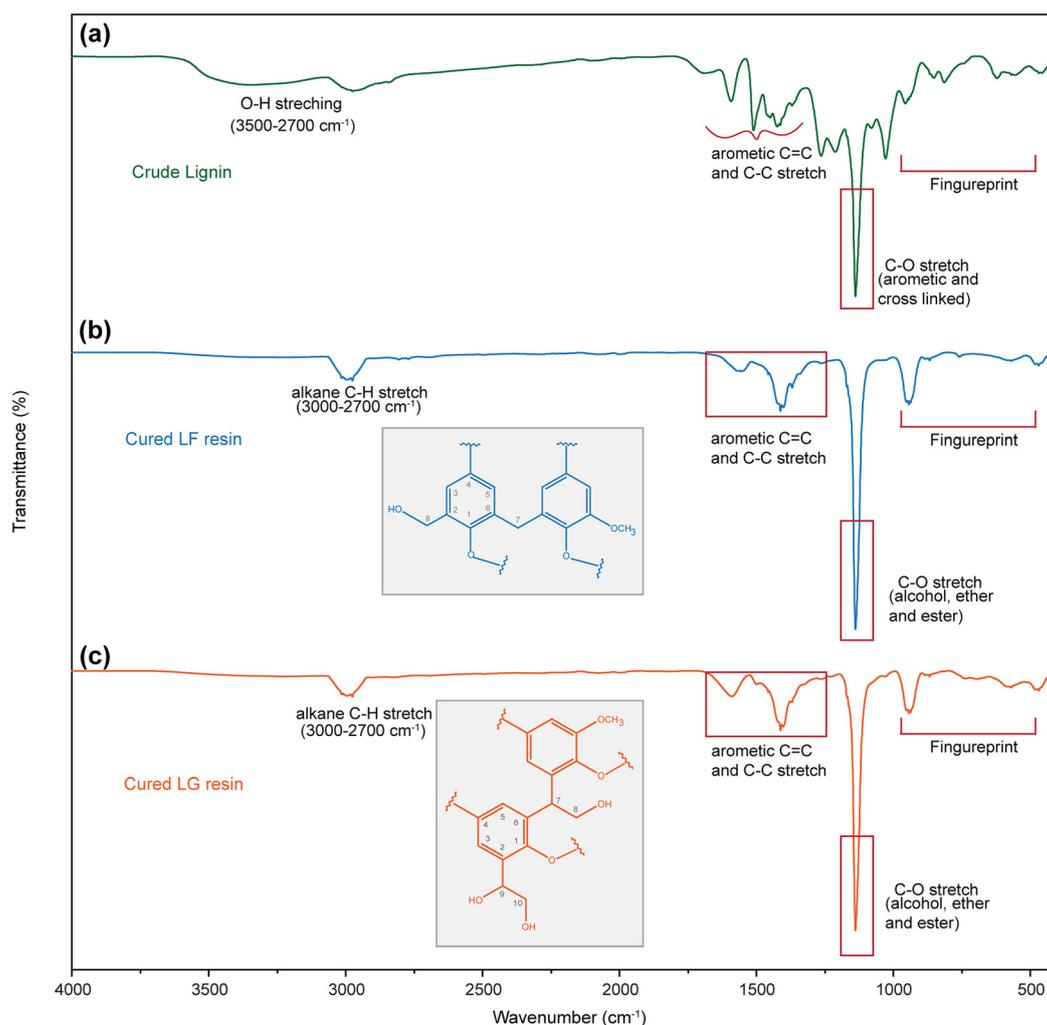
**Fig. 15** (a) FT-IR spectra of commercial lignin which contains broad O–H stretching (green spectra); (b) FT-IR spectra of LF cured resin which contain sharp C–O stretch at 1120 cm<sup>-1</sup> and significant changes in O–H and fingerprint region (blue spectra) (dimerization in LF resin in blue); (c) FT-IR spectra of LG cured resin which contain sharp C–O stretch at 1120 cm<sup>-1</sup> and significant changes in O–H and fingerprint region (red spectra) (dimerization in LG resin in orange).
