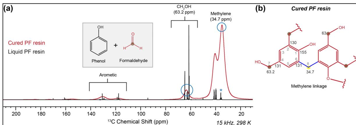
Fig. 5 (a) Comparison of liquid  $^{13}\text{C}$  NMR spectra of liquid PF resin with the  $^{13}\text{C}$ -CP MAS spectra of cured PF resin ( $\text{CH}_2\text{OH}$  at 63.2 ppm and methylene linkage at 34.7 ppm). (b) Dimer fragment of the polymeric cured PF resin, which consists of both  $\text{CH}_2\text{OH}$  group and methylene linkage (blue circles identify conversion of  $\text{CH}_2\text{OH}$  to  $\text{CH}_2$ ). Blue asterisk shows the solvent peak of  $\text{DMSO-d}_6$  at 39.5 ppm.
