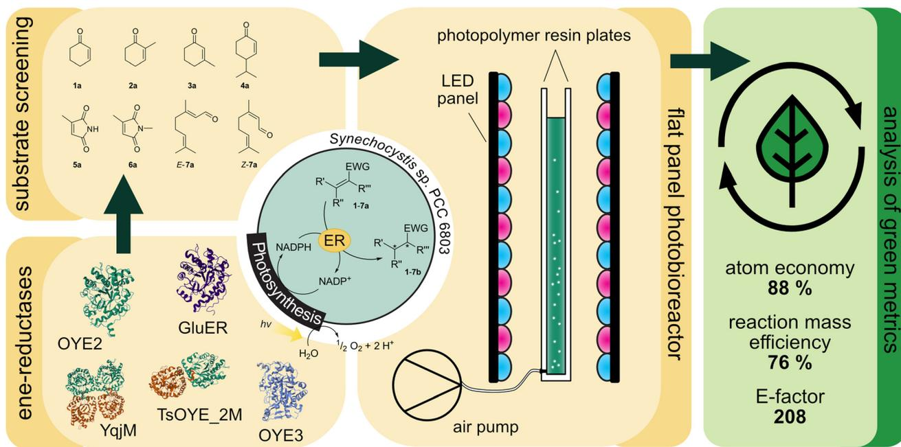
**Fig. 1** Light-driven asymmetric alkene reductions in recombinant *Synechocystis* sp. PCC 6803. Ene-reductases from different classes are produced in the cyanobacterium and the substrate scope of the strains was investigated. The best producing strains were investigated in the flat panel photobioreactor and the green metrics are analysed.
