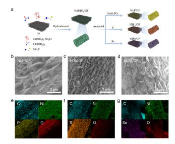
Fig. 1 (a) Schematic illustration of the synthesis route for the  $Ni_2P/NiS_2/NiSe$ . All the experimental procedures are kept the same except for the anion source. SEM images of  $Ni_2P/GF$  (b),  $NiS_2/GF$  (c) and NiSe/GF (d). Elemental mapping of  $Ni_2P/GF$  (e),  $NiS_2/GF$  (f) and NiSe/GF (g).
