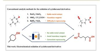
Scheme 1 Schematic comparison of 3-methyladipic acid production pathways.
