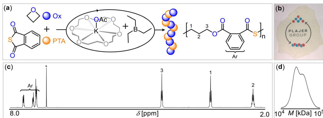
Fig. 1 (a) PTA/OX ROCOP scheme. (b) Photograph of polymer film. (c)  $^1\text{H}$  spectrum ( $\text{CDCl}_3^*$ , 400 MHz) as well as (d) gel-permeation chromatogram (GPC) of copolymer corresponding to Table 1 run #9.
