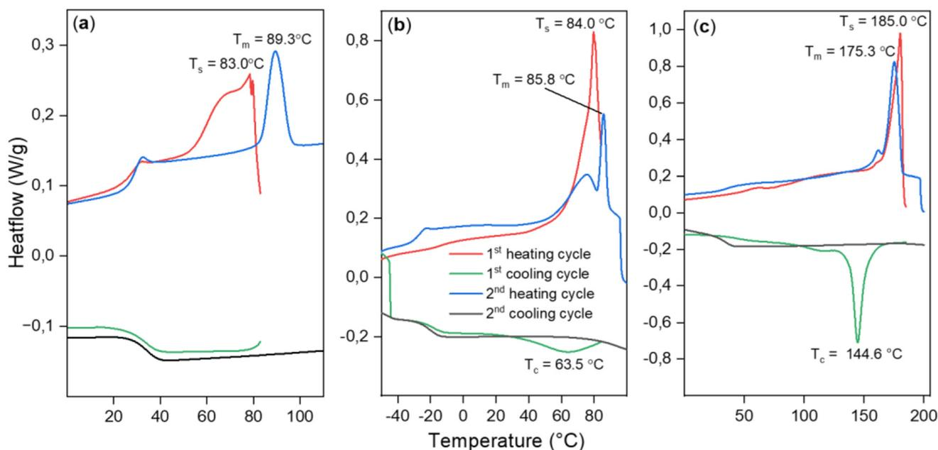
Fig. 4 DSC data showing results of self-nucleation experiments for (a) PTA/OX copolymer (Table 2, run #1), (b)  $\text{CS}_2/\text{OX}$  copolymer (Table 2, run #12), (c) PhNCS/OX copolymer (Table 2, run #8).
