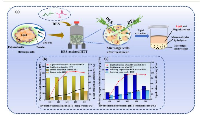
Fig. 7 Lipid extraction from microalgae using DES-HTT. (a) Flowchart of lipid extraction from microalgae via DES-HTT. (b) Lipid extraction and protein solubilisation from wet microalgae by conventional HTT and DES-HTT.<sup>101</sup> (c) Lipid extraction and reducing sugar solubilisation after the disintegration of wet microalgae by conventional HTT and DES-HTT. 101
