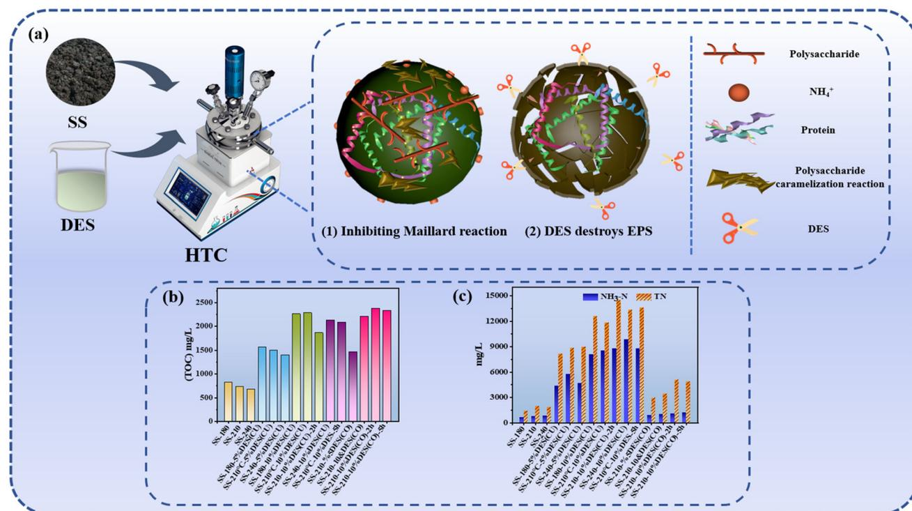
Fig. 8 Enhancing nitrogen removal from SS using DES-mediated HTC. (a) Schematic diagram of DES-mediated HTC for enhancing nitrogen removal from SS. (b) Total organic carbon (TOC) concentrations in the aqueous phase.<sup>113</sup> (c) NH<sub>3</sub>-N and total nitrogen (TN) concentrations in the aqueous phase.<sup>113</sup>
