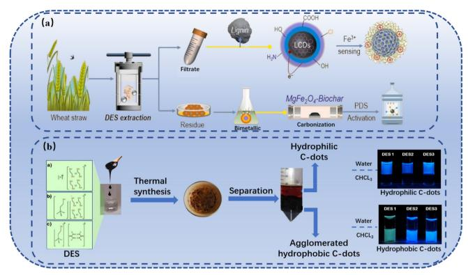
Fig. 10 The synthesis of CDs with the help of DESs. (a) Scheme for the synthesis of CDs from DES-extracted lignin *via* the DES-mediated carbonization process. <sup>137</sup> (b) Scheme for the synthesis of hydrophobic and hydrophilic CDs from molasses using DES as the reaction media. <sup>139</sup>
