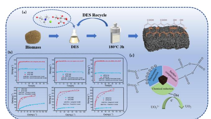
Fig. 9 Synthesis of biocarbons with rich carboxyl and phenol groups *via* DES-mediated HTC for highly efficient uranium adsorption.<sup>10</sup> (a) The scheme for functional biocarbon synthesis *via* DES-mediated HTC. (b) Uranium adsorption kinetics and isotherms for biocarbons from conventional HTC and DES-mediated HTC. (c) Uranium adsorption mechanisms for the resultant biocarbon.
