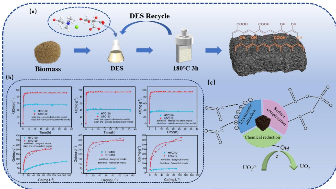
**Fig. 9** Synthesis of biocarbons with rich carboxyl and phenol groups *via* DES-mediated HTC for highly efficient uranium adsorption.<sup>10</sup> (a) The scheme for functional biocarbon synthesis *via* DES-mediated HTC. (b) Uranium adsorption kinetics and isotherms for biocarbons from conventional HTC and DES-mediated HTC. (c) Uranium adsorption mechanisms for the resultant biocarbon.
