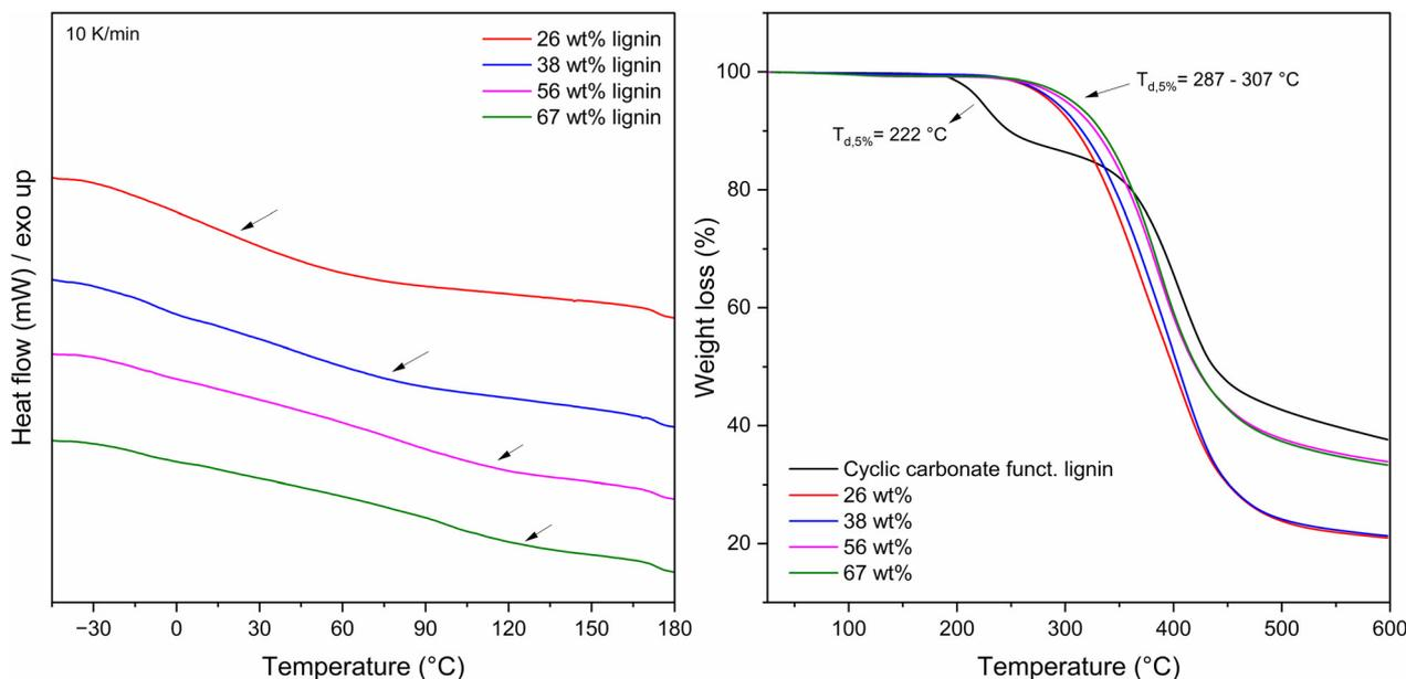
Fig. 4 Left: DSC thermograms of thermosets with different lignin weight percentages (compare Table 3), right: TGA decomposition curves for the CCFL (black) and the thermosets with different lignin weight percentages.
