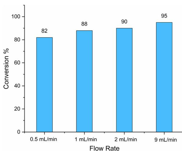
**Fig. 2** Conversions of HOSO via thiol-ene reaction in flow at different flow rates after 3 h. To evaluate the conversion, a 100 μL sample was taken at different reaction times and <sup>1</sup>H-NMR was recorded. Reactions in isopropanol with a flow rate 0.5 ml min<sup>-1</sup>, 1 ml min<sup>-1</sup>, 2 ml min<sup>-1</sup> and 9 ml min<sup>-1</sup> were performed.
