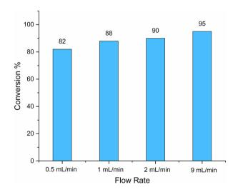
Fig. 2 Conversions of HOSO via thiol—ene reaction in flow at different flow rates after 3 h. To evaluate the conversion, a 100  $\mu$ L sample was taken at different reaction times and  $^{1}$ H-NMR was recorded. Reactions in isopropanol with a flow rate 0.5 mL min $^{-1}$ , 1 mL min $^{-1}$ , 2 ml min $^{-1}$  and 9 mL min $^{-1}$  were performed.
