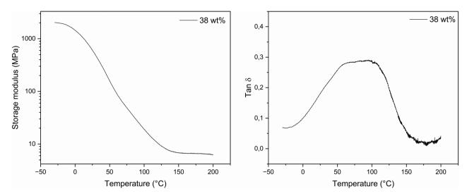
Fig. 5 Left: representative curve of the storage modulus (E') curve against temperature for the 38 wt% lignin content thermoset. Right: representative curve of the tan ( $\delta$ ) curve against temperature for the 38 wt% lignin content thermoset.
