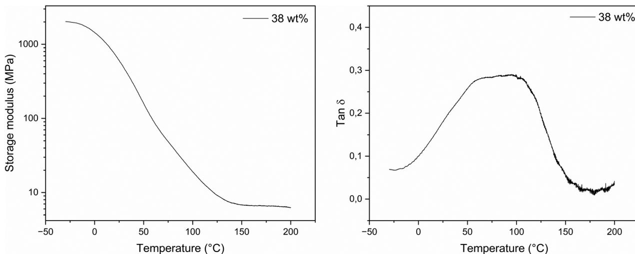
Fig. 5 Left: representative curve of the storage modulus ( $E'$ ) curve against temperature for the 38 wt% lignin content thermoset. Right: representative curve of the  $\tan(\delta)$  curve against temperature for the 38 wt% lignin content thermoset.
