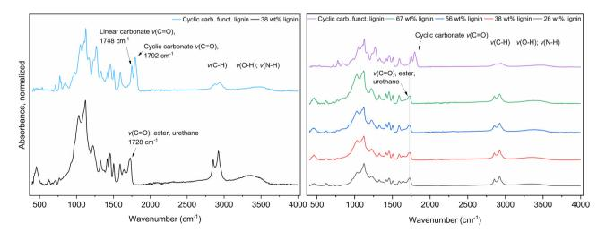
Fig. 3 Left: overlayed IR spectra of CCFL (blue, top) and the thermoset with 38 wt% lignin content (Table 4, entry 2, black, bottom). Right: overlay of IR spectra of CCFL (violet, top) and the thermosets with different lignin compositions (see Table 4). Relevant signal changes are highlighted.
