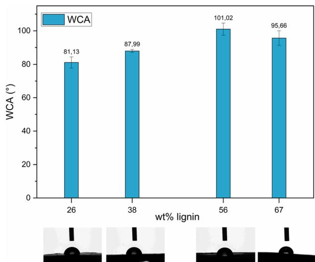
**Fig. 6** Water contact angle measurements for thermosets with different lignin composition. Measurements were performed 5 times per sample to ensure reproducibility and average values are reported, as well as measurement errors.
