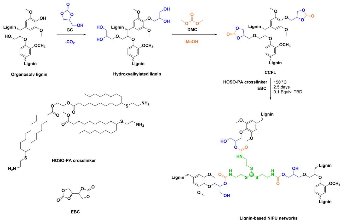
**Scheme 2** General reaction scheme for lignin functionalization to achieve CCFL, and subsequent reaction with EBC and crosslinker PA to form NIPU networks. For simplicity, only the main reactions are shown, for further details and discussion see ESI.†
