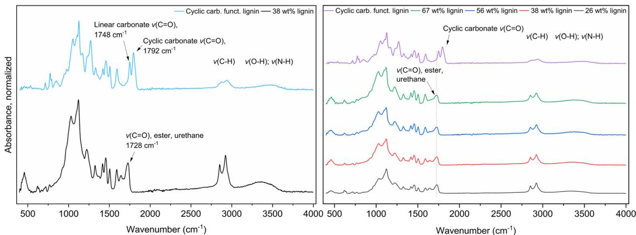
**Fig. 3** Left: overlaid IR spectra of **CCFL** (blue, top) and the thermoset with 38 wt% lignin content (Table 4, entry 2, black, bottom). Right: overlay of IR spectra of **CCFL** (violet, top) and the thermosets with different lignin compositions (see Table 4). Relevant signal changes are highlighted.
