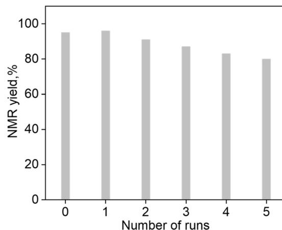
**Fig. 7** Catalyst recycling for the reductive amidation of PLA with 4-fluoronitrobenzene. Reaction conditions: 0.5 mmol of 4-fluoronitrobenzene, 30 mg of poly(lactic acid), 20 mg of catalyst (3 mol% Ni), 20 bar H<sub>2</sub>, 0.8 mL of toluene, 0.2 mL of H<sub>2</sub>O, 140 °C, 24 h. Yields were determined by NMR using acetonitrile as the standard.
