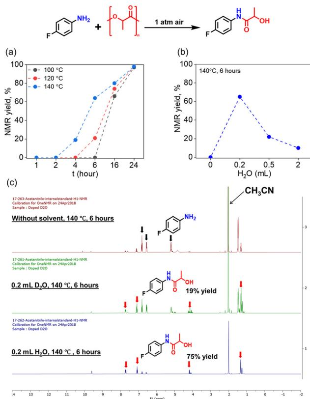
**Fig. 4** The effect of (a) temperature and (b)  $\text{H}_2\text{O}$  volume on the product yield. (c) The corresponding NMR spectra. Reaction conditions: 2 mmol 4-fluoroaniline, 117 mg PLA, 100–140  $^{\circ}\text{C}$ , no catalysts, 0–2 mL  $\text{H}_2\text{O}$  or  $\text{D}_2\text{O}$ . Yields were determined by NMR using acetonitrile as standard.
