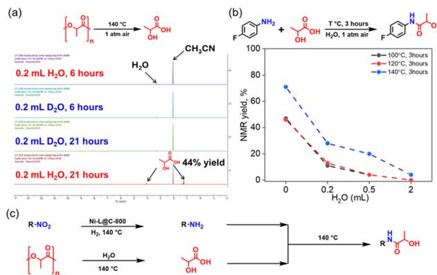
**Fig. 5** The function of  $\text{H}_2\text{O}$  in PLA amidation. (a) Reaction conditions: 117 mg of PLA, solvent, no catalysts, 140  $^{\circ}\text{C}$ , 6–21 h. (b) Reaction conditions: 2 mmol of 4-fluoroaniline, 1.624 mmol of lactic acid, no catalysts. Yields were determined by NMR using acetonitrile as the standard. (c) Proposed mechanisms.
