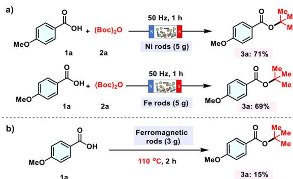
**Scheme 4** The influence of metal in steel needles on the experimental results. Conditions: **1a**: 0.5 mmol, **2a**: 1.0 mmol, high temperature and pressure resistant reaction tube: 10 mL, Ni rods, Fe rods: 5 g, 1.0 × 5.0 mm, reaction time: 1 h, frequency: 50 Hz.
