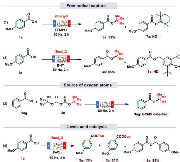
**Scheme 5** Mechanism exploration experiment. Conditions: **1a**: 0.5 mmol,  $(\text{Boc})_2\text{O}$ : 1.0 mmol, TEMPO: 1.5 mmol, BHT: 1.5 mmol,  $\text{FeCl}_2$ : 20 mmol%, high temperature and pressure resistant reaction tube: 10 mL, ferromagnetic rods: SUS304, 5 g,  $0.3 \times 5.0$  mm, reaction time: 2 h, frequency: 50 Hz. ND: not detected.
