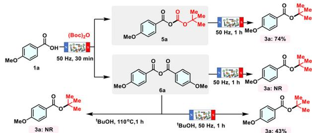
**Scheme 3** Control experiment. Conditions: **1a**: 0.5 mmol, **2a**: 1.0 mmol, **5a**: 0.5 mmol, **6a**: 0.5 mmol, high temperature and pressure resistant reaction tube: 10 mL, ferromagnetic rods: SUS304, 5 g, 0.3 × 5.0 mm, reaction time: 2 h, frequency: 50 Hz, *t*-BuOH: 1.0 mL. NR: no reaction.
