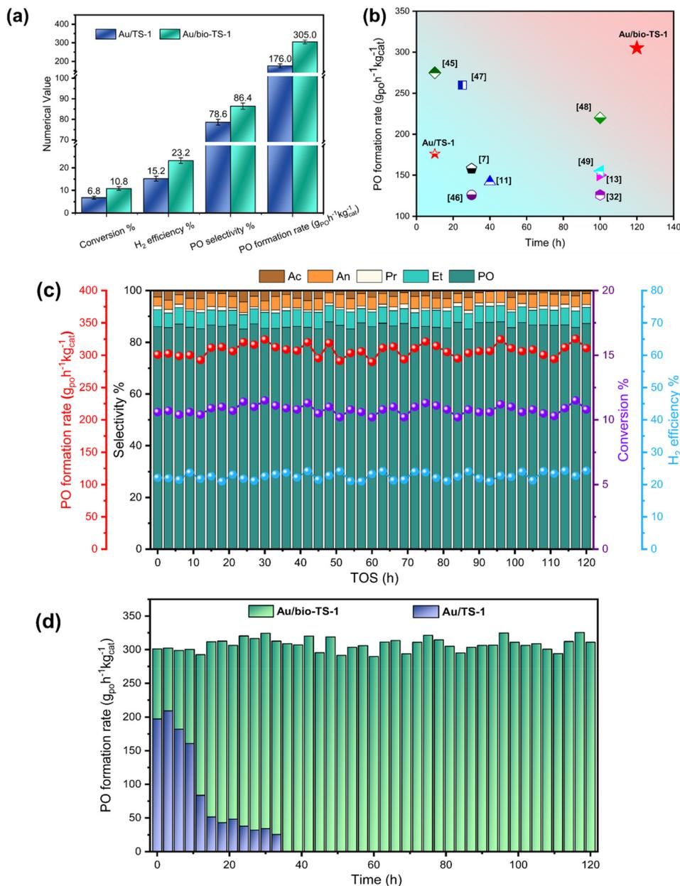
**Fig. 4** (a) Catalytic performance and (b) comparison of performance between this work and recent work. (c) Stability test results of the Au/bio-TS-1 catalysts. (d) PO formation rate of Au/bio-TS-1 and Au/TS-1 catalysts (reaction conditions: H<sub>2</sub>/O<sub>2</sub>/C<sub>3</sub>H<sub>6</sub>/Ar = 1/1/1/7, 200 °C, GHSV = 14 000 mL g<sup>-1</sup> h<sup>-1</sup>).
