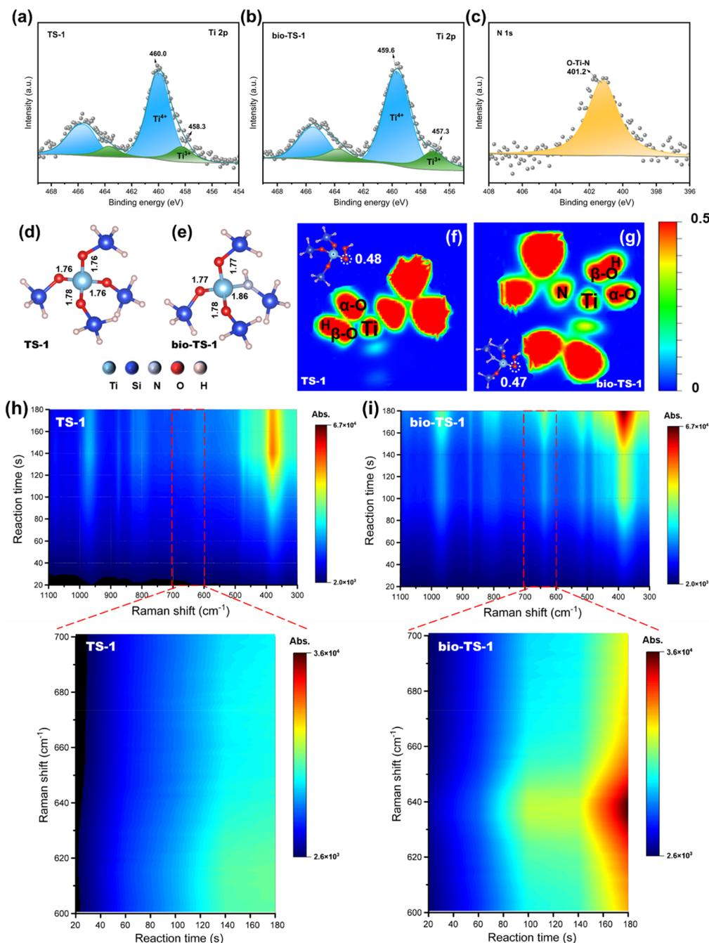
**Fig. 3** (a and b) XPS spectra for Ti 2p of TS-1 and bio-TS-1. (c) N 1s of bio-TS-1. Optimized geometry and electronic localized functions (ELF) of Ti-OOH with (d and f) TS-1 and (e and g) bio-TS-1. Quasi *in situ* Raman spectra of (h) TS-1 and (i) bio-TS-1 at different exposure times.
