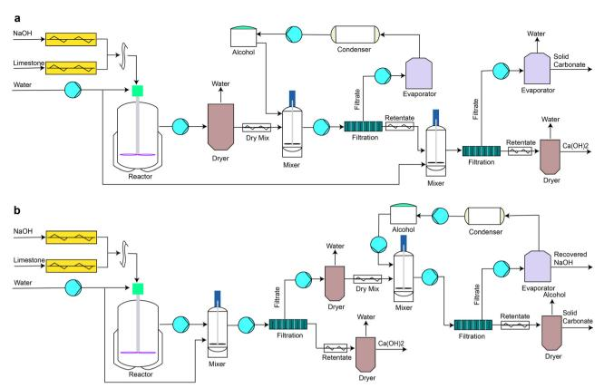
Fig. 1 Flow diagrams of the two processes (a: process A, b: process B). In process "A", the unreacted NaOH after the anion exchange reaction is separated first before separating the Na<sub>2</sub>CO<sub>3</sub> from the mixture of Ca-containing compounds, Ca(OH)<sub>2</sub> and CaCO<sub>3</sub>. In process "B", the Ca-containing compounds are separated from the mixture after adding excess water to remove/dissolve both NaOH and Na $_2$ CO $_5$ . <sup>15</sup>
