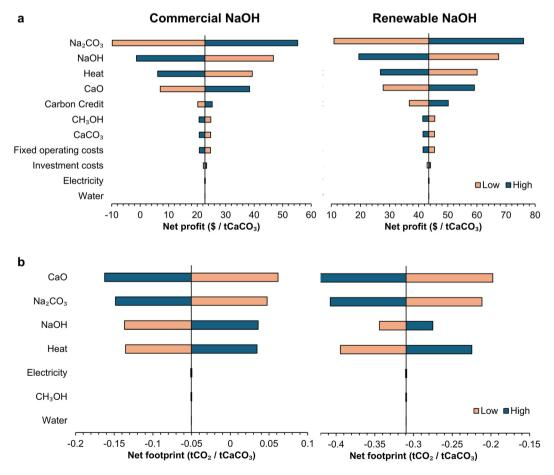
Fig. 8 Effects of different factors on the profitability (a) and  $CO_2$  emissions (b) of the anion-exchange process. The sensitivity of the profit and  $CO_2$  footprint was calculated when the cost and  $CO_2$  footprints were lowered ("low") or increased ("high") by 20%. The analysis was performed for process B for the mix design Experiment ID 19 (water: 30.7, NaOH: 30.9, and  $CaCO_3$ : 38.4 wt%) for both renewable and commercial NaOH cases.
