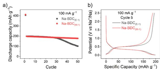
**Fig. 1** (a) Discharge capacity and (b) galvanostatic charge/discharge curves for Na-BDC materials (5th cycle) cycled between 0.01–2.5 V at a current rate of 100 mA g<sup>-1</sup>.
