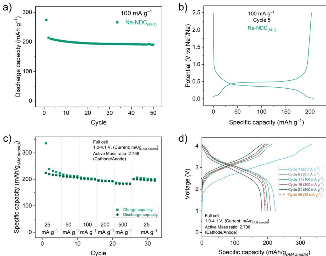
**Fig. 2** (a) Discharge capacity and (b) galvanostatic charge/discharge curves for Na-NDC materials (5<sup>th</sup> cycle) cycled between 0.01–2.5 V at a current rate of 100 mA g<sup>-1</sup>. Rate performance for full-cell prepared using Na-NDC<sub>(M-1)</sub> as anode, (c) discharge capacity at different current rates, cycled five times at every step, and (d) corresponding charge/discharge curves for first cycle of every step.
