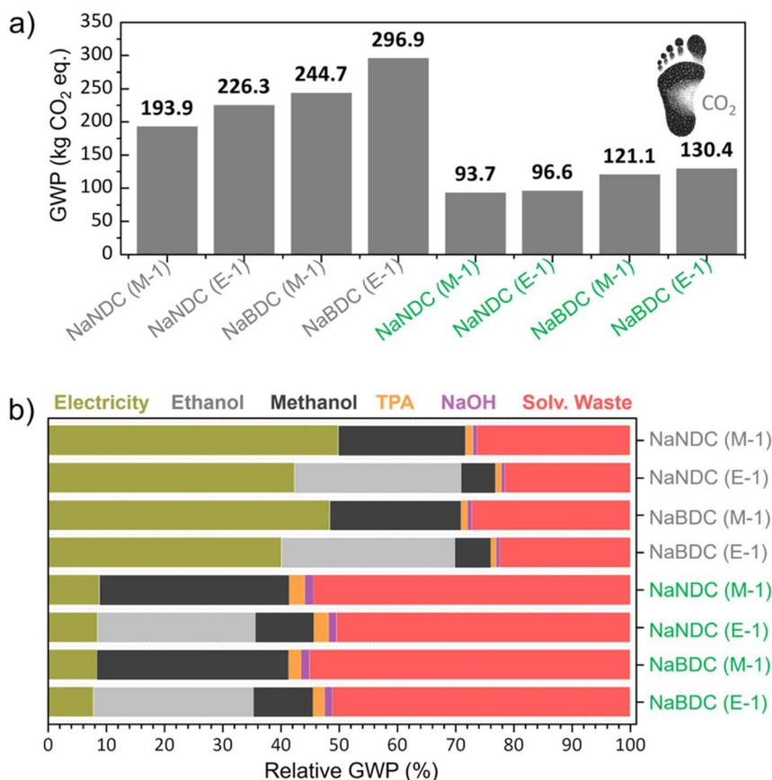
**Fig. 3** Global warming potential (GWP) of Na-NDC and Na-BDC. (a) Absolute value and (b) relative CO<sub>2</sub> share depending on process input/outputs. Green labels represent syntheses performed utilising a renewable energy grid ("market for electricity, low voltage, renewable energy products | electricity, low voltage, renewable energy products | Cutoff, U – CH"). TPA = terephthalic acid/H<sub>2</sub>BDC.
