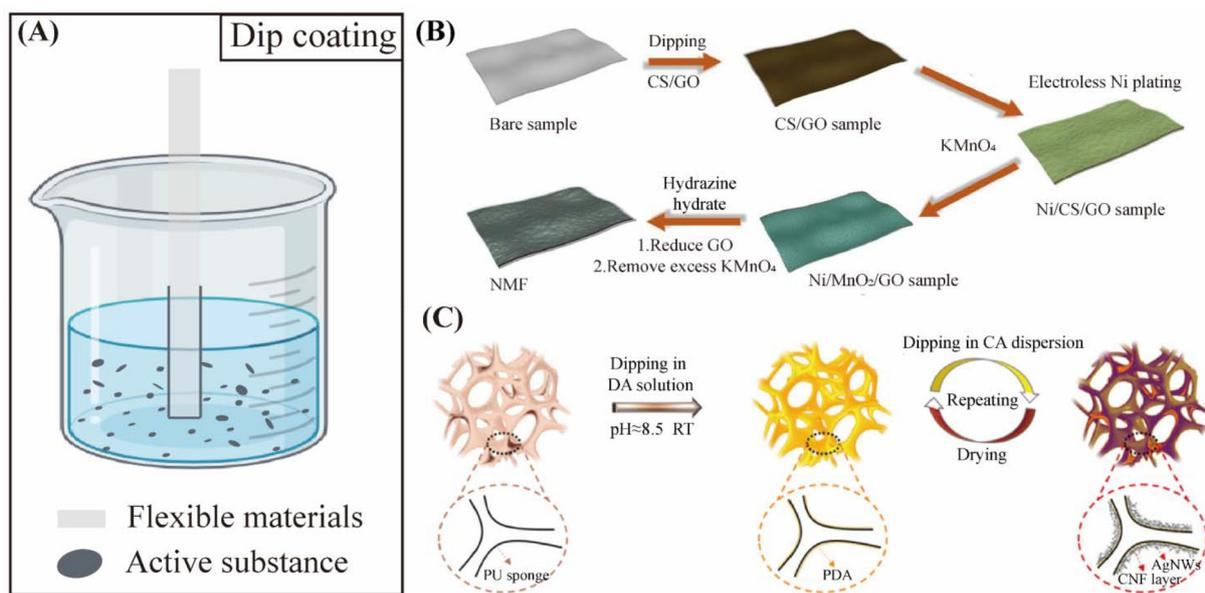
**Fig. 6** (A) Schematic of the manufacturing principle of the dip-coated sensor. (B) Preparation of flexible sensors by chemical nickel plating after dip-coating of fibers with an active substance. Reprinted with permission from ref. 116. Copyright (2019) American Chemical Society. (C) Schematic illustration for the preparation of conductive CA@PU sponge. Reprinted with permission from ref. 117. Copyright (2019) American Chemical Society.
