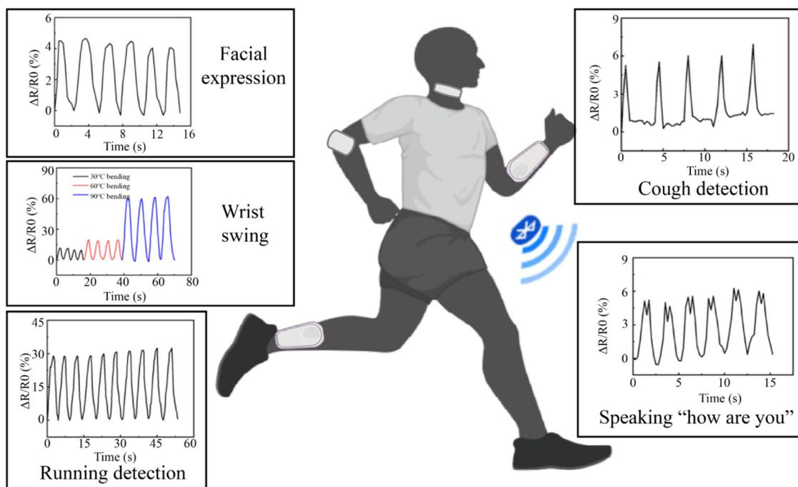
**Fig. 8** Wearable flexible sensors detect a person's coughs, facial expressions, wrist swings at different bending, running, and speaking "how are you". Reprinted with permission from ref. 133. Copyright (2021) Elsevier.
