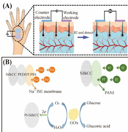
**Fig. 7** (A) Structure and working principle of the two-electrode non-invasive blood glucose sensor. Schematic to show extraction of ISF by the RI process. Reprinted with permission from ref. 130. Copyright (2021) Elsevier. (B) Schematic diagram showing the working mechanisms of  $\text{Na}^+$ , pH, and glucose sensors. Reprinted with permission from ref. 132. Copyright (2023) Elsevier.
