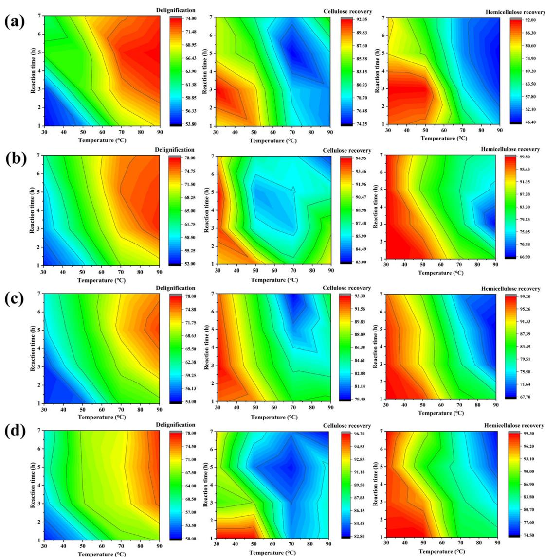
Fig. 5 Effect of the reaction temperature and time on delignification, cellulose and hemicellulose recovery: (a) TMAH-urea; (b) TMAH-MEA; (c) TMAH-lysine and (d) TMAH-imidazole.
