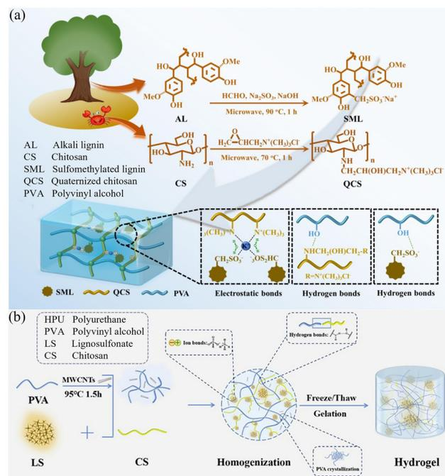
**Fig. 4** Different interactions in lignin-based hydrogels prepared by the physical crosslinking method.<sup>87,109</sup> (a) Electrostatic bonds and hydrogen bonds. [Reproduced from ref. 109 with permission from Elsevier, copyright of 2024.] (b) Ionic bonds and hydrogen bonds. [Reproduced from ref. 87 with permission from American Chemical Society, copyright of 2023.]
