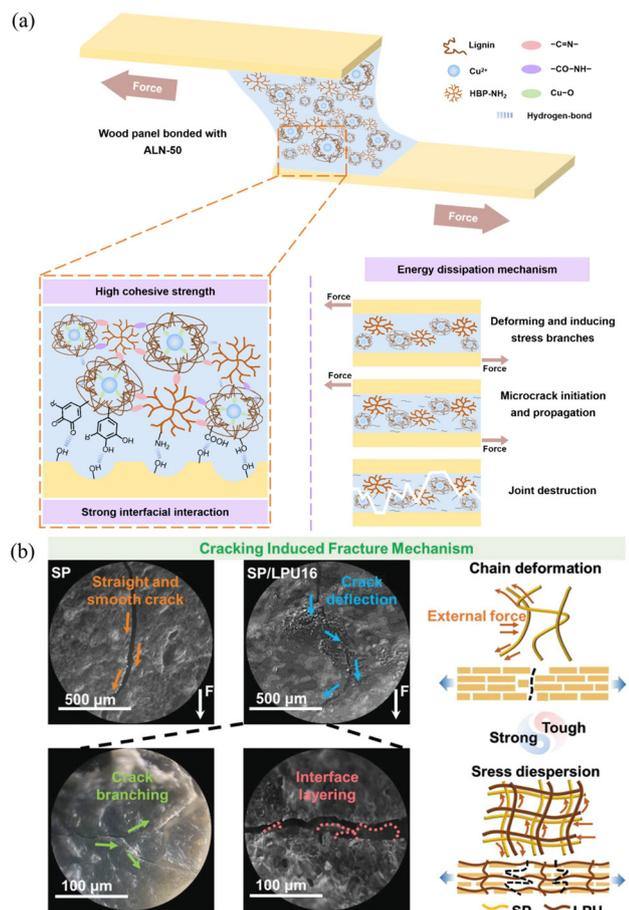
**Fig. 10** (a) Strengthening and toughening mechanism of a lignin-based adhesive.<sup>136</sup> [Reproduced from ref. 136 with permission from Elsevier, copyright of 2024.] (b) Cross-sectional analysis of an SP-based adhesive for fracture.<sup>140</sup> [Reproduced from ref. 140 with permission from Wiley, copyright of 2024.]
