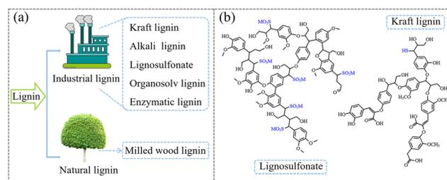
Fig. 2 (a) Different types of lignin. (b) The structure of lignosulfonate and kraft lignin.<sup>47,48</sup> [Reproduced from ref. 47 and 48 with permission from Wiley, copyright of 2022.]
