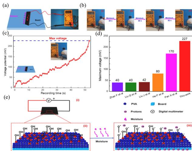
**Fig. 8** (a) Schematic diagram of the lignin reinforced PVA hydrogel-based moist-electric generator (LRP-HMEG) and (b) voltage output of LRP-HMEG under continuous moisture flow. (c) The effect of moisture duration on voltage. (d) Comparison of electric power generation of LRP-HMEG and other moist-electric generators. (e) Mechanism of the moist-electric generator.<sup>84</sup> [Reproduced from ref. 84 with permission from Elsevier, copyright of 2021.]
