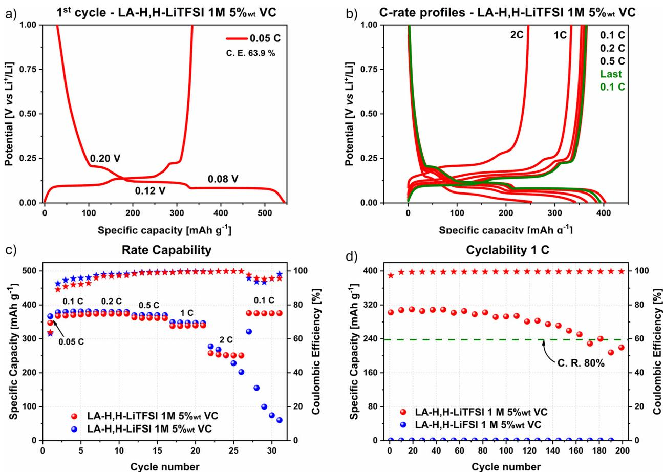
**Fig. 2** GR galvanostatic charge/discharge profile with LA-H,H-LiTFSI 1 M 5 wt% VC of (a) 1<sup>st</sup> cycle at 0.05C, and (b) profiles at different current densities over capability test. (c) Results from rate capability (5 cycles per each current density), and (d) cyclability (200 cycles at 1C). C. E.: coulombic efficiency. C. R.: capacity retention.
