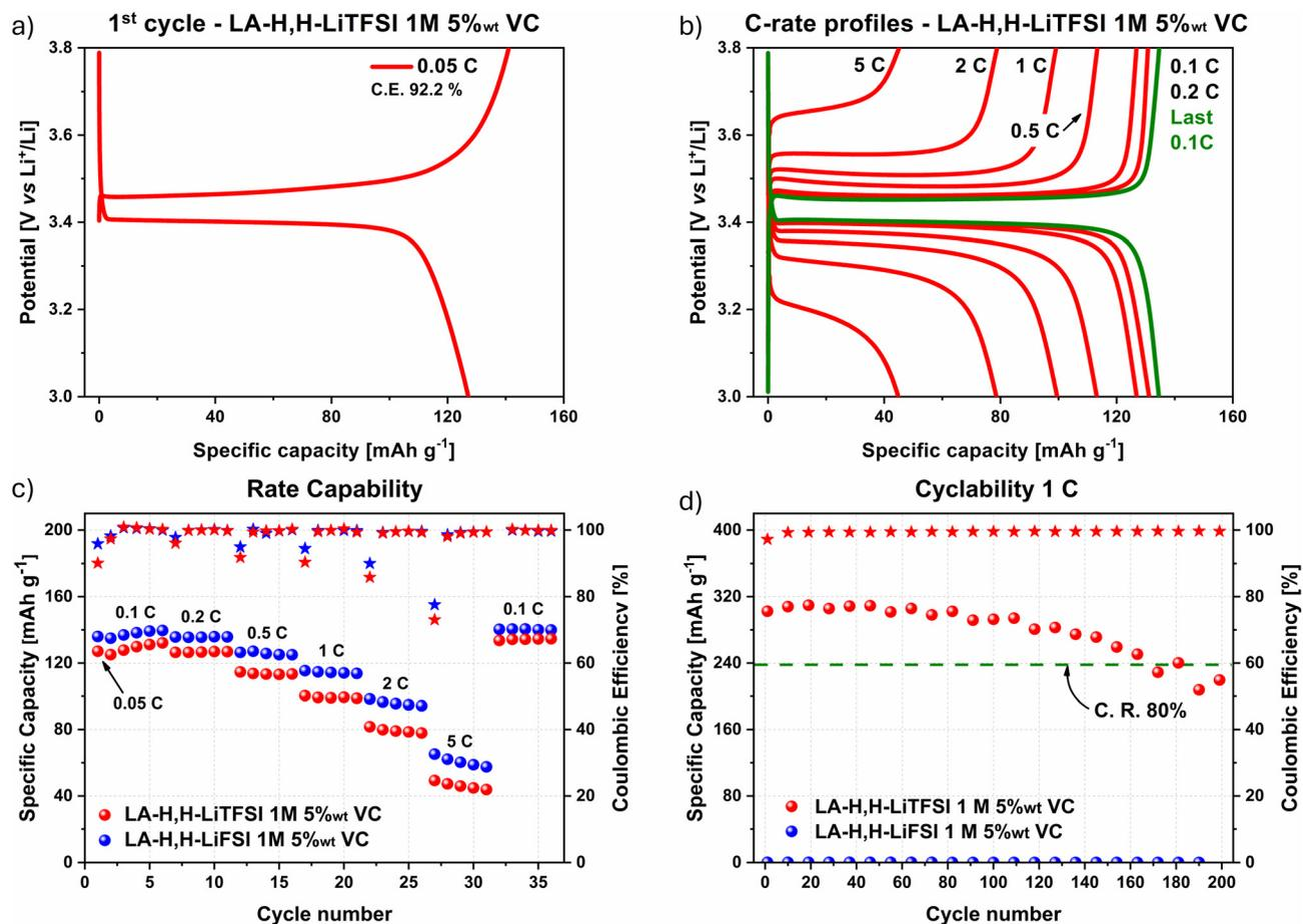
Fig. 3 LFP galvanostatic charge/discharge profile with LA-H,H-LiTFSI 1 M 5 wt% VC of (a) 1<sup>st</sup> cycle at 0.05C, and (b) profiles at different current densities over capability test. (c) Results from rate capability (5 cycles per each current density), and (d) cyclability (200 cycles at 1C). C. E.: coulombic Efficiency. C. R.: capacity retention.
