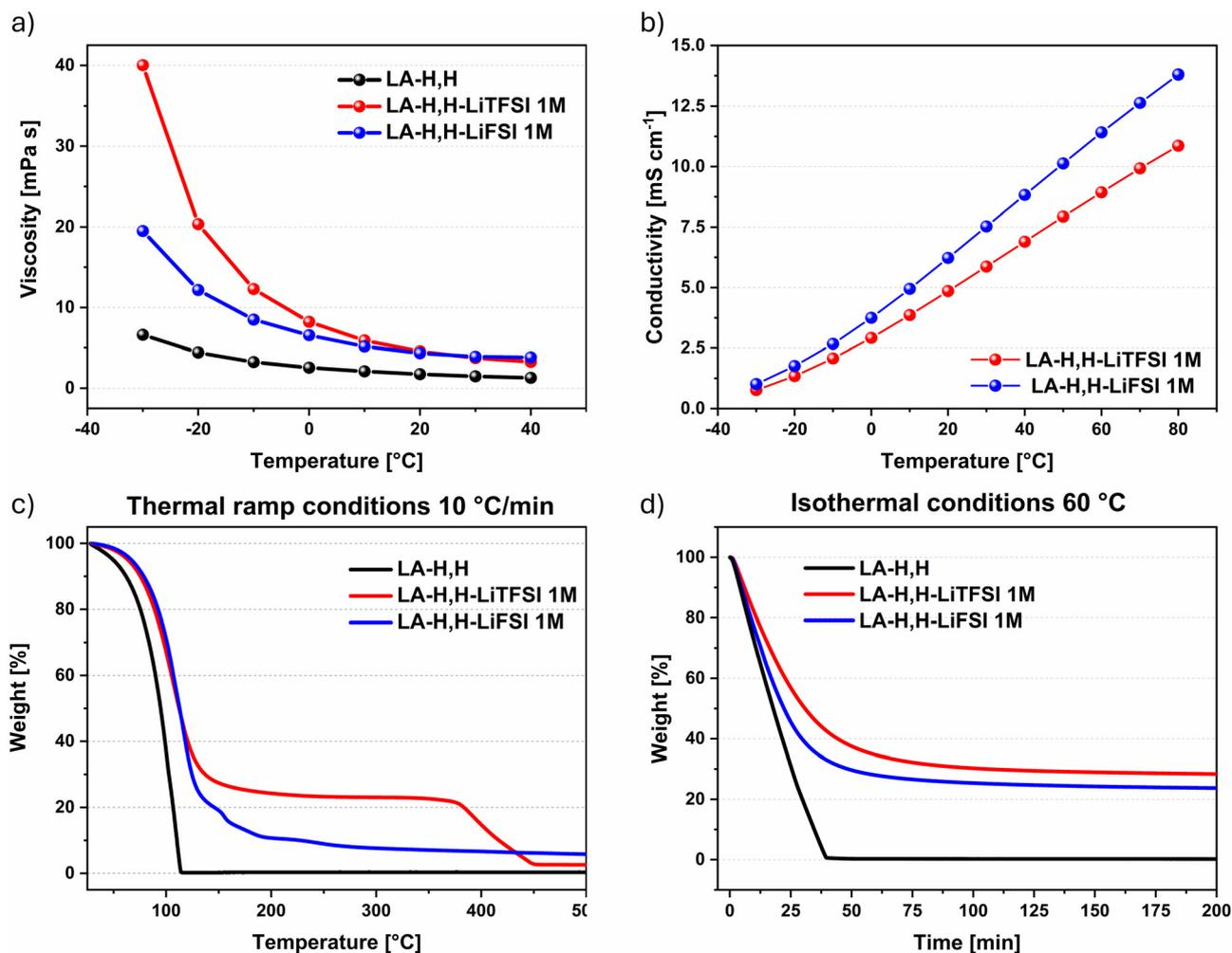
Fig. 1 (a) Viscosity measured from  $-30$  °C to  $40$  °C, and (b) conductivity measured from  $-30$  °C to  $80$  °C, (c) dynamic TGA from  $30$  °C to  $550$  °C, and (d) isothermal TGA at  $60$  °C.
