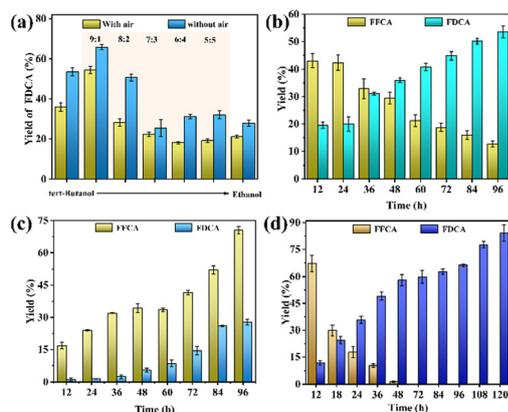
**Fig. 3** The performances of a one-pot photo-enzymatic catalysis system for the selective oxidation of DFF into FDCA. (a) The impact of *tert*-butanol and ethanol ratio in buffer towards the FDCA production under aeration. Samples were taken after 96 h of reactions. The time course of the FDCA production from DFF by photo-enzymatic catalysis in buffer consisted of (b) pure *tert*-butanol, (c) pure ethanol, and (d) 9 : 1 of *tert*-butanol/ethanol.
