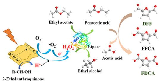
**Fig. 6** Proposed reaction mechanism of the one-pot photo-enzymatic catalysis for selective oxidation of DFF into FDCA. In the depiction, white represents hydrogen atoms, red represents oxygen atoms, and gray represents carbon atoms.
