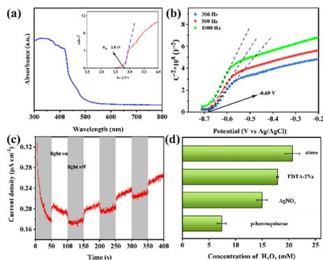
**Fig. 4** Characterization of the photocatalytic performances by 2-ethylantraquinone and free radical scavenging experiments. (a) UV-vis DRS, (b) Mott-Schottky (M-S), and (c) transient photocurrent responses. (d)  $\text{H}_2\text{O}_2$  production using 2-ethylantraquinone as a photocatalyst in the presence of reactive species scavengers.
