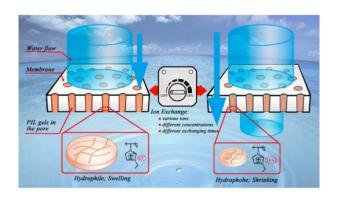
Fig. 3 Salt-responsive PES membranes integrated with anion-sensitive poly(ionic liquid) (PIL) gels prepared with methacrylatoethyl trimethyl ammonium chloride ([MTA][CI]). Reproduced from ref. 78 with permission from American Chemical Society, copyright 2017.
