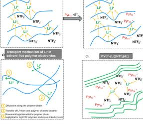
Fig. 4 (a) Li<sup>+</sup>-ion coordination and (c) transport mechanisms in PEObased, binary polymer electrolytes. Li<sup>+</sup>-ion coordination in ternary polymer electrolytes containing (b) active polymers (e.g. PEO) and (d) inactive polymers (e.g. PVdF). Adapted from ref. 96 with permission from John Wiley & Sons, copyright 2015.
