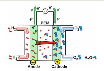
Fig. 6 Schematic representation of a proton exchange membrane fuel cell. 109
