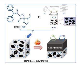
Schematic representation of the synthesis and burning mechanism of flame-retardant RPUFs compounded with IL-EG/DPES. Reproduced from ref. 117 with permission from Multidisciplinary Digital Publishing Institute, copyright 2020.
