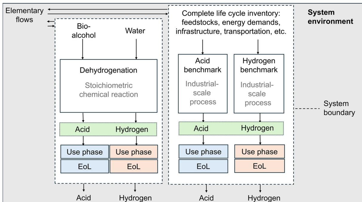
**Fig. 1** System boundaries in a cradle-to-grave analysis of the dehydrogenation route and the benchmark with system expansion for the production of hydrogen and acid. The functional unit is highlighted in green. The use phase and end of life (EoL) of the acid (blue) and the hydrogen (orange) are equal for identical products.
