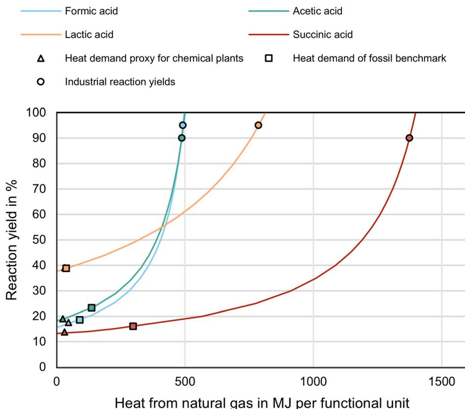
Fig. 5 Trade-off for dehydrogenation routes between reaction yield and allowed heat demand to arrive at zero environmental potential for the investigated dehydrogenation routes in a fossil benchmark scenario in the climate change impact category. The triangles represent heat demands based on a proxy for chemical plants.<sup>57</sup> The squares represent the heat demands of the fossil benchmarks. The circles represent industrial reaction yields.
