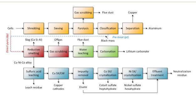
Fig. 2 Simplified process flowsheet in scenarios *dp* (red, green, and blue units) and *pt* (yellow, red, green, and blue units). Units are classified into pre-treatment (yellow), pyrometallurgical processing (red), flue dust treatment for lithium recovery (green), and hydrometallurgical alloy refining (blue).
