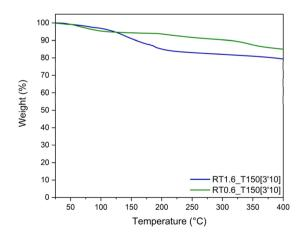
Fig. 10 Thermogravimetric analyses of the resins obtained by extrusion with different TPA-to-resorcinol molar ratios. The extrusion temperature was set to 150 °C with a flow rate of 1 kg h $^{-1}$  and a screw speed of 100 rpm. The thermograms were recorded at 10 °C min $^{-1}$  under an inert atmosphere.
