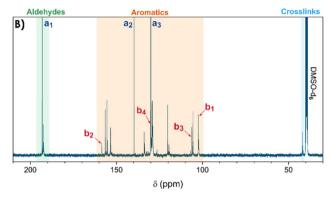
Fig. 1 NMR spectra of the resin synthesized by reactive extrusion with a TPA-to-resorcinol molar ratio of 1.6 (RT1.6\_T150[3'10]). The extrusion temperature was set to 150  $^{\circ}$ C with a flow rate of 1 kg  $h^{-1}$  and a screw speed of 100 rpm. (A) <sup>1</sup>H-NMR; (B) <sup>13</sup>C-NMR (DMSO-d<sub>6</sub>/298 K).
