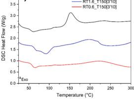
Fig. 9 DSC thermograms of resorcinol—TPA formulations with different TPA-to-resorcinol molar ratios. (A) DSC thermograms of the resorcinol—TPA formulations prior to the extrusion; (B) DSC thermograms of the synthesized resins by extrusion at 150 °C, 100 rpm and a flow rate of  $1 \text{ kg h}^{-1}$ .
