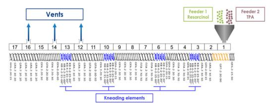
Fig. 13 Twin-screw profile.
