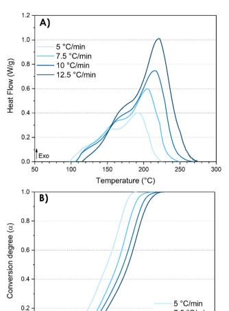
Fig. 6 DSC analyses of the pristine system resorcinol—TPA (TPA-to-resorcinol molar ratio of 1.6) before extrusion. (A) DSC thermograms after baseline corrections; (B) nonisothermal kinetic profiles.
