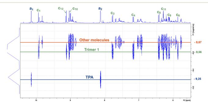
Fig. 2 2D DOSY map of the resin synthesized by reactive extrusion with a TPA-to-resorcinol molar ratio of 1.6. The extrusion temperature was set to 150 °C with a flow rate of 1 kg h<sup>-1</sup> and a screw speed of 100 rpm (RT1.6\_T150[3'10]). Diffusion time  $\Delta$  = 0.15 s and gradient pulse length  $\delta$  = 2600 μs. Solvent: DMSO-d<sub>6</sub> at 298K.
