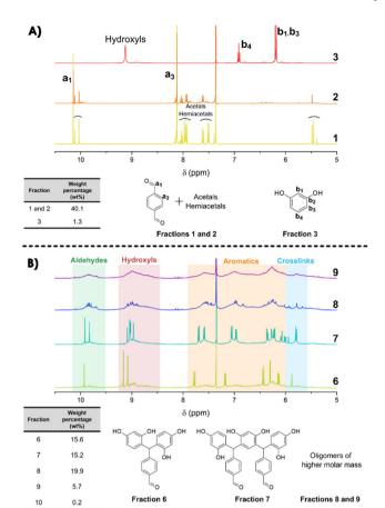
Fig. 4 <sup>1</sup>H-NMR spectra (DMSO-d<sub>6</sub>) and weight distribution of the main isolated fractions recovered by flash chromatography of the resin synthesized by extrusion (RT1.6\_T150[3'10]). For more clarity, fractions 4, 5 and 10 (2.8% of the total weight) are not presented in this figure. (A) Fractions 1 to 3 of the residual monomers; (B) fractions 6 to 9 of the oligomers synthesized.
