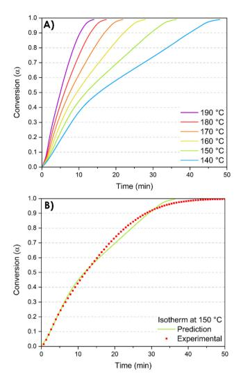
Fig. 8 Isothermal prediction curves. (A) Isothermal predictions at different temperatures; (B) comparison of predicted and experimentally measured isothermal kinetic profiles at 150 °C.
