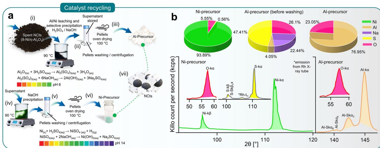
**Fig. 4** Recycling of spent NCTs. (a) Schematics (steps i–vii) elaborating the recycling method of Al and Ni from spent Ni/η-Al<sub>2</sub>O<sub>3</sub> NCTs through acid leaching and selective NaOH precipitation (pH 0–14). (b) XRF spectroscopy showing elemental concentration (%) in Al and Ni precursors recovered from spent Ni/η-Al<sub>2</sub>O<sub>3</sub> NCTs (top) and characteristic XRF peaks related to Ni, Al, S and O (bottom).
