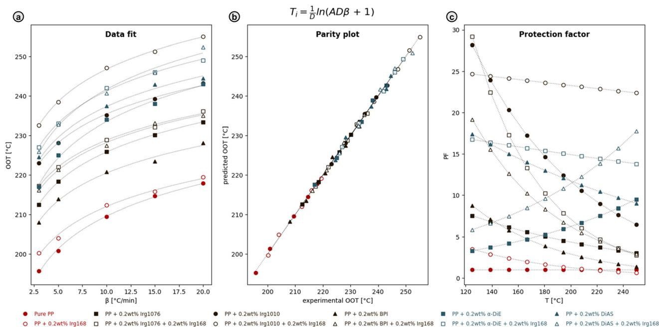
**Fig. 11** (a) Experimental and fitted dependencies of the onset oxidation temperatures (OOT) on the heating rates  $\beta$ , for pure PP and PP with added antioxidants, employing  $k(T_i) = A_k e^{DT}$  (eqn (3) from ESI M9<sup>†</sup>). Data points corresponding to samples with added heat stabilizer, Irg 168, are given as open symbols. (b) Parity plot of predicted and experimental OOT. (c) Dependence of PP protection factor (PF) on temperature.
