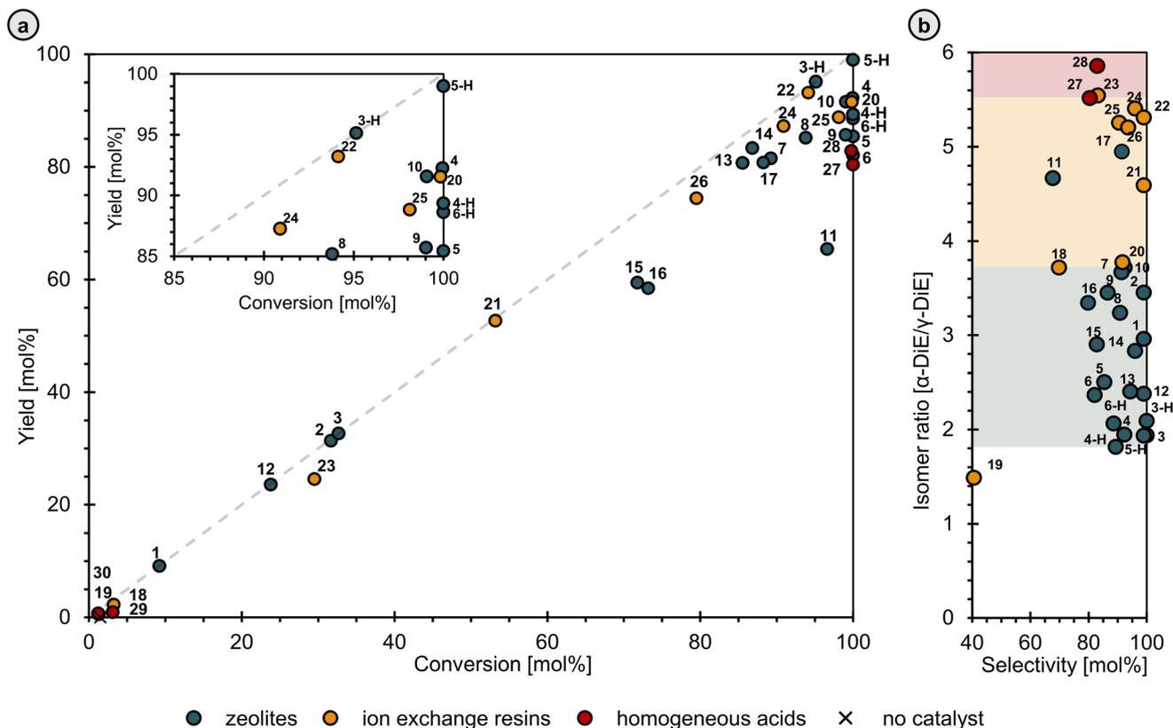
**Fig. 3** DiE synthesis with different catalysts. (a) total yield (mol%) of DiE in function of IE conversion (mol%) for different catalysts (with zoomed insert). Grey dotted line refers to 100% selectivity. (b) Isomer ratio [ $\alpha$ -DiE/ $\gamma$ -DiE] in function of selectivity (mol%). Reaction conditions: 1 mmol IE, 0.1 mmol  $H^+$ , 2.5 mL *o*-xyl, 80 °C, 4 h, 750 rpm.
