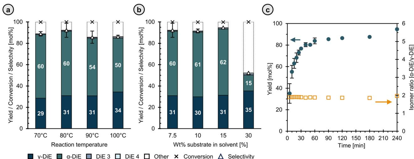
**Fig. 6** (a) Yield, conversion, and selectivity (mol%) for reaction with CBV720 at different temperatures (4 h, 7.5 wt% IE). (b) Yield, conversion, and selectivity (mol%) and the  $\alpha/\gamma$  diastereoisomer ratio at different points in time, employing the ideal reaction conditions (15 wt% IE, 80 °C). Reaction conditions: 1 mmol IE, 0.1 mmol  $H^+$  (CBV720), *o*-xyl, 750 rpm.
