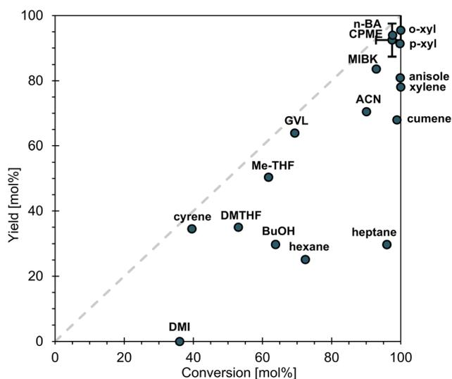
Fig. 5 Total yield of DiE in function of IE conversion in different solvents. Grey dotted line refers to 100% selectivity. Reaction conditions: 1 mmol IE, 0.1 mmol H<sup>+</sup> (CBV720), 2.5 mL solvent, 80 °C, 4 h, 750 rpm.
