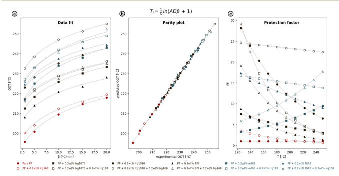
Fig. 11 (a) Experimental and fitted dependencies of the onset oxidation temperatures (OOT) on the heating rates  $\beta$ , for pure PP and PP with added antioxidants, employing  $k(T_i) = A_{ij}e^{DT}$  (eqn (3) from ESI M9†). Data points corresponding to samples with added heat stabilizer, Irq 168, are given as open symbols. (b) Parity plot of predicted and experimental OOT. (c) Dependence of PP protection factor (PF) on temperature.
