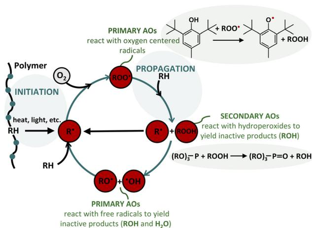
**Fig. 1** Polymer degradation process. Schematic representation of the polymer degradation process (blue) and the protective role of primary and secondary antioxidants (green). Figure adapted from ref. 4 and 5.
