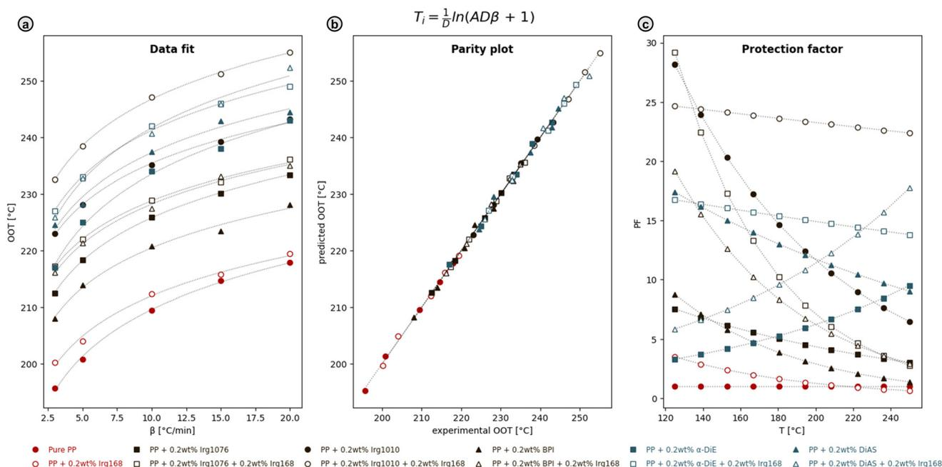
**Fig. 11** (a) Experimental and fitted dependencies of the onset oxidation temperatures (OOT) on the heating rates  $\beta$ , for pure PP and PP with added antioxidants, employing  $k(T_i) = A_k e^{DT}$  (eqn (3) from ESI M9†). Data points corresponding to samples with added heat stabilizer, Irg 168, are given as open symbols. (b) Parity plot of predicted and experimental OOT. (c) Dependence of PP protection factor (PF) on temperature.
