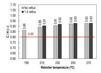
**Fig. 10** C/H ratio of the heavy fraction. Red line: C/H of the starting TPO.
