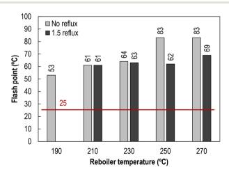
Fig. 11 Flash point of the heavy fraction. Red line: flash point of the starting TPO.
