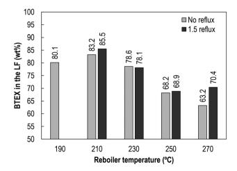
Fig. 8 BTEX concentration in the light fraction.
