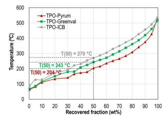
Fig. 4 Simulated distillation curve (ASTM D2887).
