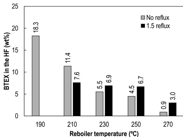
Fig. 9 BTEX concentration in the heavy fraction.
