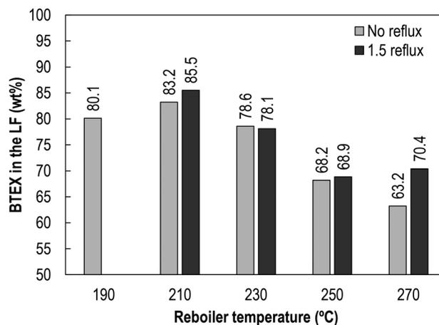
Fig. 8 BTEX concentration in the light fraction.
