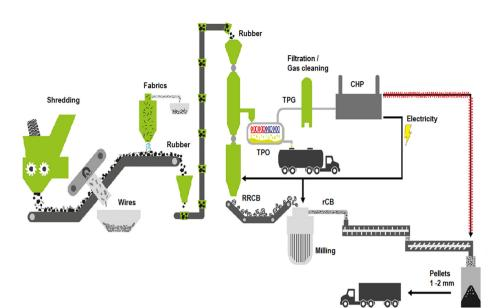
Fig. 2 General overview of the Pyrum's process for pyrolysis of ELT.
