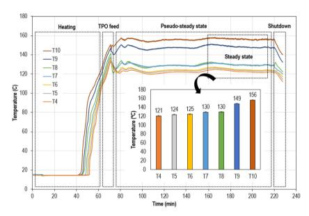
Fig. 6 Temperature profiles at 210 °C with no reflux (run # 2).
