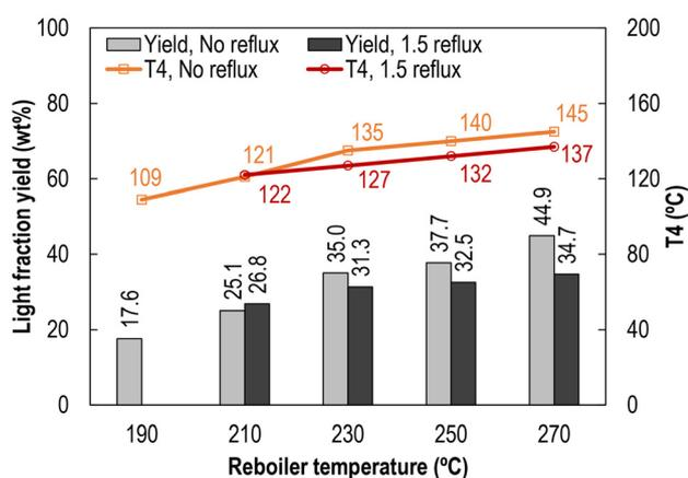
Fig. 7 Light fraction yield and T4 temperature.
