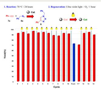
Fig. 4 Reuse and reactivation of multifunctional systems based on RB-Cu(OAc)<sub>2</sub>-TS-SILLP-5a for the reaction between 7a and 8b. 0.2 M azide: alkyne (1:1) in acetonitrile, 0.7% mol copper catalyst, 24 hours and 70 °C. Blue bar: result obtained for the fresh Cu(OAc)<sub>2</sub>-TS-SILLP-5a at 4 hours and 70 °C. \* 11<sup>th</sup> reuse at 4 hours and 70 °C performed after reactivation.
