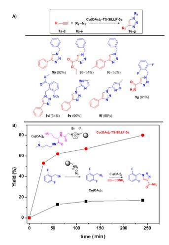
Fig. 2 (A) Scope of the catalyst Cu(OAc)<sub>2</sub>-TS-SILLP-5a for different alkynes and azides. (B) Yield of Rufinamide (9g) vs. time for immobilized Cu(OAc)<sub>2</sub>-TS-SILLP-5a and Cu(OAc)<sub>2</sub> as a homogeneous catalyst (reaction conditions: 0.2 M azide: alkyne (1:1) in acetonitrile, 1.5% mol copper catalyst, 70 °C).
